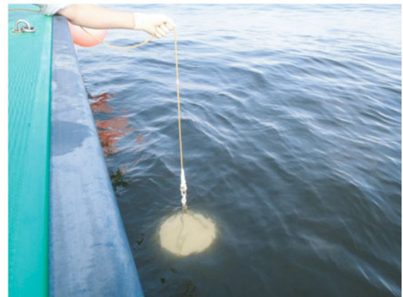
Fig. 2.34 Monitoring points and a snapshot of transparency observation (Furukawa and Ishimaru 2012)
