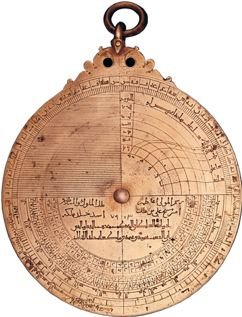
Figure 8.10. The back of a brass astrolabe made by Badr ibn ‘Abdallah ca. 1130 probably in Baghdad. 18.8 × 13.4 cm. Note the Persian writing and the absence of an alidade sighting bar. Courtesy of the Adler Planetarium & Astronomy Museum, Chicago, Illinois, A-84.
