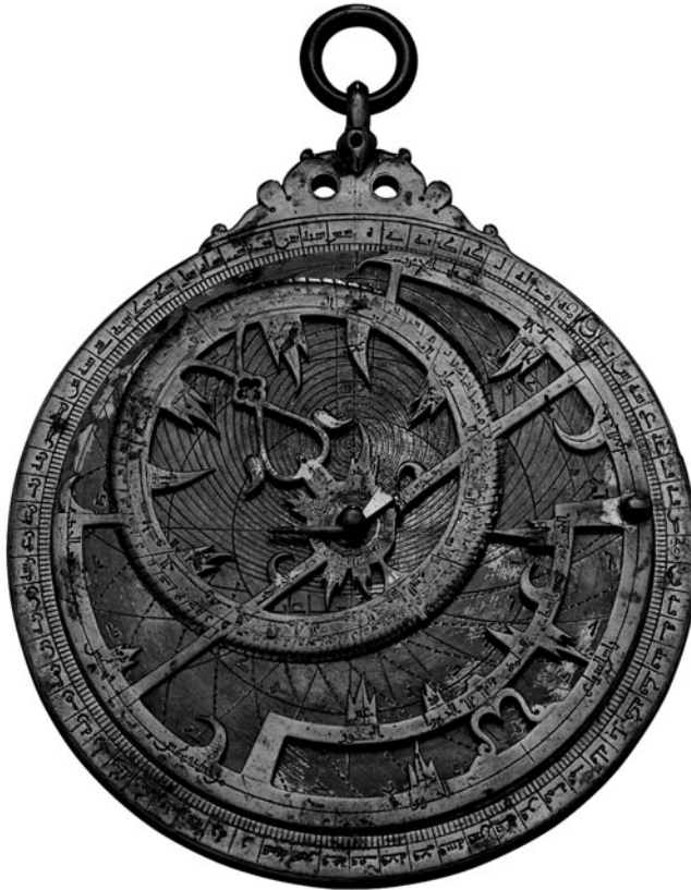
Figure 8.9. The front of a brass astrolabe made by Badr ibn ‘Abdallah ca. 1130 probably in Baghdad. 18.8 \times 13.4 cm. Note the rete star map and the tympan engraved with circles of altitude for the latitude of Persia. Courtesy of the Adler Planetarium & Astronomy Museum, Chicago, Illinois, A-84. See also Color Section 3.
