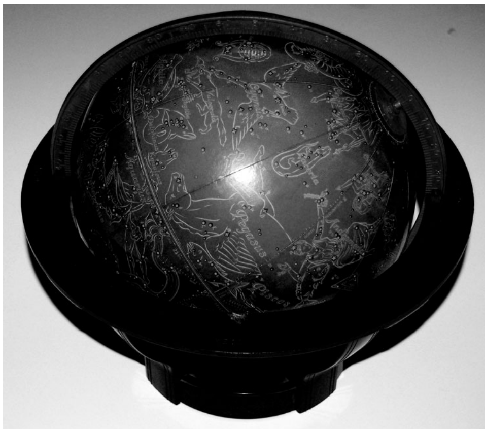
Figure 8.1. 9-inch celestial globe on a Bakelite stand, produced by Rand McNally in 1936. Note the stars in yellow (see Color Section 3), the mirror-reversed constellation images in light blue, and the dark blue background, which simulates the night sky. Note also the movable, vertical calibrated meridian ring on which the globe is attached; the hour ring near the north equatorial pole of the globe; and the fixed horizon circle that is connected to the base. Copyright Rand McNally & Co. Reproduced with permission, R.L.07-S-22.
