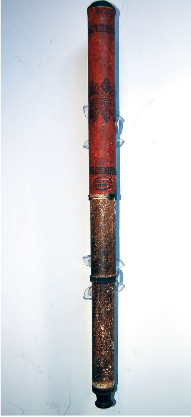
Figure 8.16. Small spyglass-type refracting telescope made by Semitecolo, a well-known Venetian telescope maker, ca. 1800. It is made out of pasteboard, with bony rings separating each section. The main tube is 25.5 cm long. Note the beautiful floral and Greek key design and the screw-on eyepiece cap.
