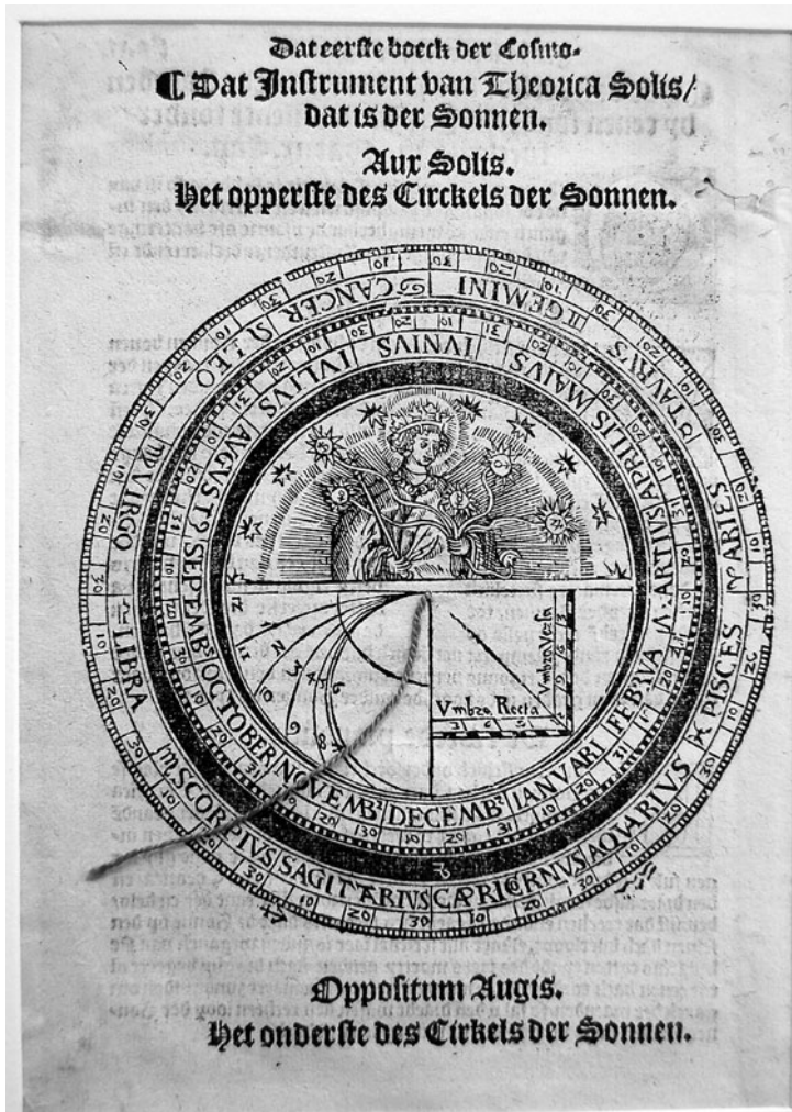
Figure 3.15. Page from the 1533 edition of Apian's Cosmographia . 12.4 cm dia. Note the volvelle (i.e., a printed calculating device—see Section 8.2), which here is similar in appearance to an astrolabe, with zodiac and month circles on the periphery, unequal hour lines in the center left, and a shadow square in the center right. There is a string attached to the center that serves as a pointer.
