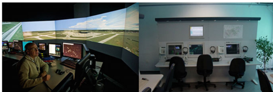
Fig. 4 Simulation venues. Aerodrome control simulator on the left , radar control simulator on the right
