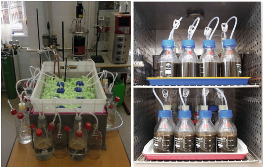
Fig. 6 Batch reactor systems used during the experiments. Source own photo
