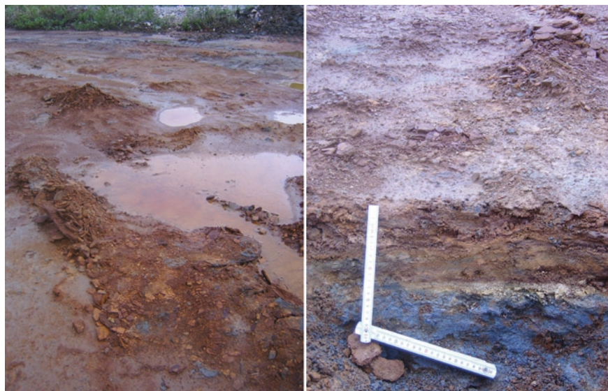
Fig. 5.18 Bare soil surface ( left ) and soil profile ( right ) of a copper mining area in Tongling, China; the blue colour is due to high concentration of arsenic and cyanides
