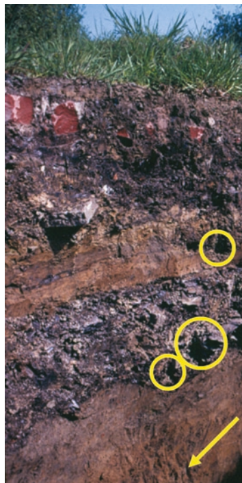
Fig. 7.4 Soil profile in Gelsenkirchen, Germany consisting of industrial construction debris in which tar residues ( circles ) exist; the tar is moving downward using channels left by earthworms ( arrow )
