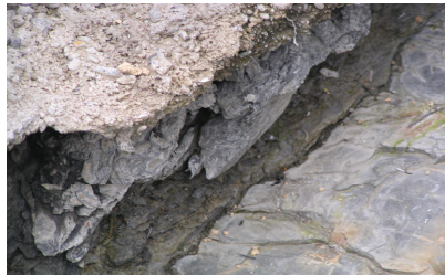
Fig.2. The muddy sandwich in the terrain of the landslide(0+460)
