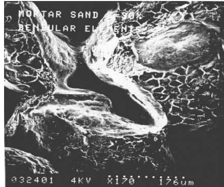
FIG. 7. Vesicular character and honey comb structure of foam.
