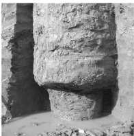
FIG. 4. Photo of T-shaped cement-soil deep mixing column
