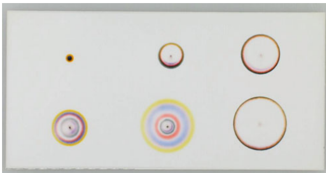
Fig. 4.6 Using spot tests to optimize the separation of a CAMAG dye mixture (on silica gel) with 35 \mu\text{L} each of cyclohexane, diethyl ether, tert -butyl methyl ether, methylene chloride, toluene, and ethyl acetate (from top left to bottom right ). Methylene chloride and toluene show the best separation
