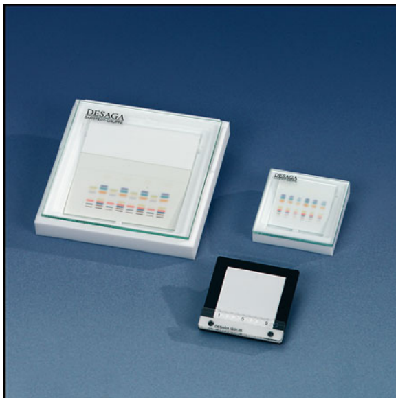
Fig. 6.8 H-chambers (according to Kraus) with a 10 \times 10 cm and a 5 \times 5 cm HPTLC plate (With permission of DESAGA, Heidelberg, Germany.)
