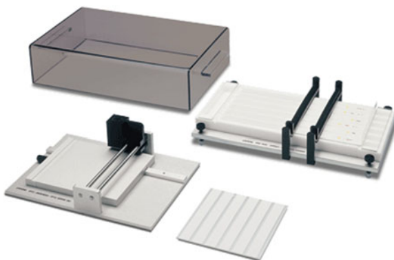
Fig. 6.7 A Vario-KS-Chamber (top, right) with scoring unit. For pre-conditioning, the layer is placed over the main chamber body on the left side where six trays are scratched out. For development, the plate is slid to the right side with no vapour below (With permission from CAMAG, Muttensz, Switzerland.)
