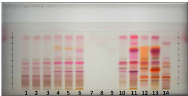
Fig. 7.7 Separation of ethyl acetate extracted Iceland moss ( CETRARIA ISLANDICA ) on HPTLC Si 60 F 254 with acetone, methanol, formic acid, toluene (5+5+10+80, v/v), chamber saturation, stained with anisaldehyde reagent
