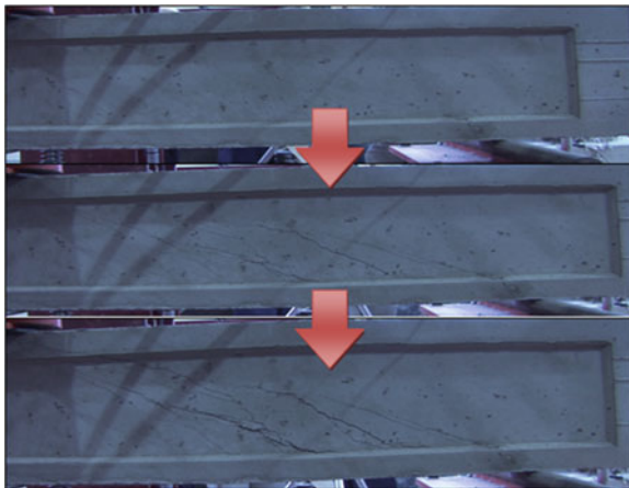
Fig. 6.8 Shear crack evolution (failure mode III)
