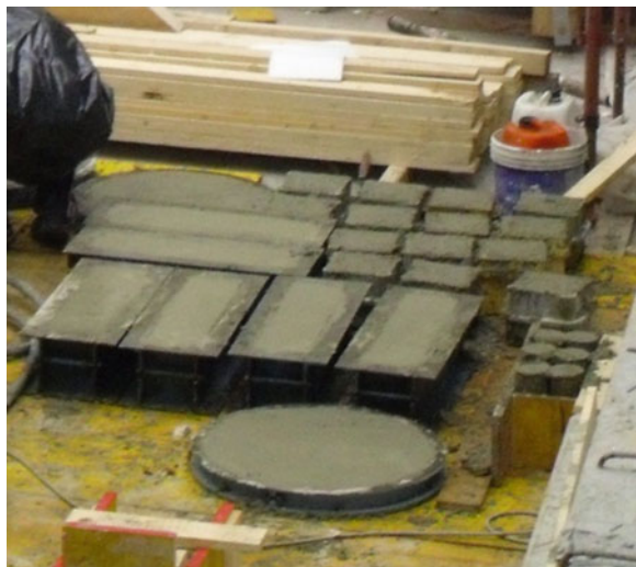
Fig. 5.3 Round panel and cylinder, cubic and prismatic specimens just produced
