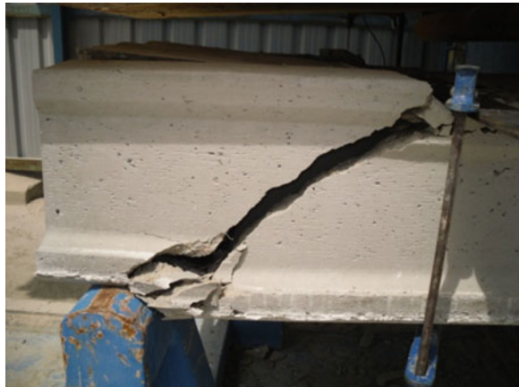
Fig. 7.10 Crack caused by tension shear and anchorage failure simultaneously
