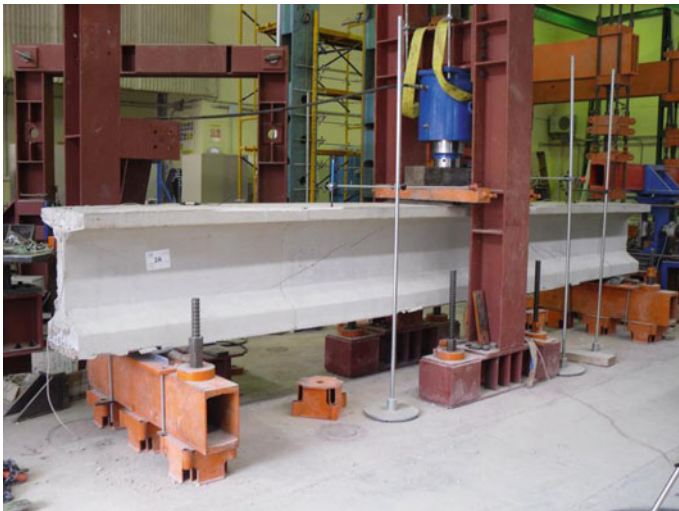
Fig. 4.5 Beam during shear test
