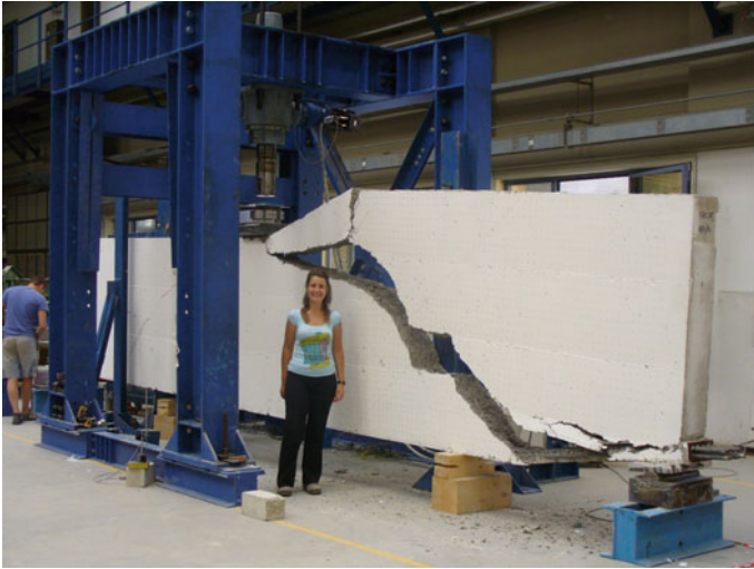
Fig. 5.15 Beam H1500-FRC75 after its failure
