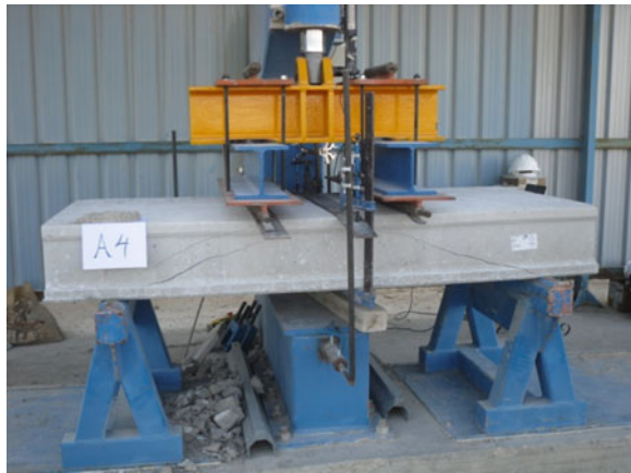
Fig. 7.5 Test set-up. Shear diagonal tension failure
