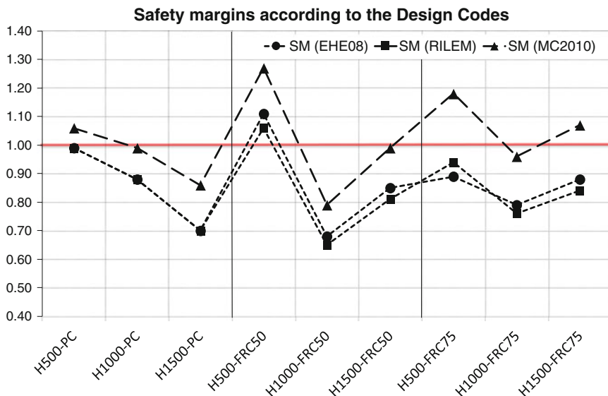
Fig. 5.35 Safety margin (SM) = V_{\text{test}}/V_{\text{theo}} without safety factors
