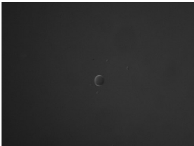
Fig. 10.15 Stereomicroscope image of silicone oil droplet in water. Silicone oil has a distinctive appearance that is quite different than the appearance of air bubbles. The silicone droplet is easier to see directly on the stereomicroscope than it is to photograph. The oil droplets are generally in motion and so difficult to keep in focus for the photomicrograph (image size = 3.4 \times 2.5 mm)
