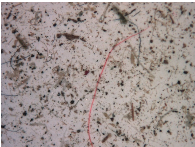
Fig. 10.2 Dust particles observed with a stereomicroscope. This sample was collected by brushing dust from a surface in a garage used for woodworking and gardening. It shows a wide variety of different particle types and is a useful sample for practicing techniques of particle identification (image size = 3.4 \times 2.5 mm)
