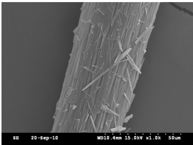
Fig. 4.2 Caffeine hydrate crystal. This photomicrograph illustrates the easy interpretation of SEM images. We see a near three-dimensional appearance of a bundle of crystals with other crystals lying on the surface. The appearance of the image seems to accord well with our sense of sight in the natural world. (Image size = 122 \times 99 \mu\text{m} )
