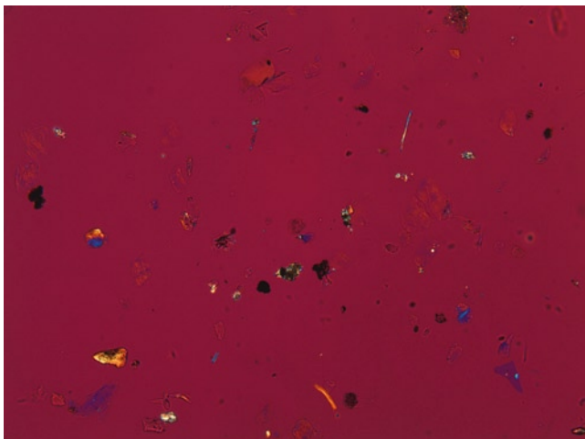
Fig. 10.3 Dust particles by polarized light microscopy. This image shows a wide variety of different particles by PLM. Such a sample would be indicative of a cleaning process malfunction since there are so many environmental samples. Classifying the particles by morphology and by interference colors suffices for this type of sample (image size = 700 \times 520 \mu\text{m} )
