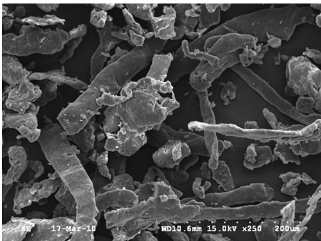
Fig. 4.13 SEM Photomicrograph of Hydroxy Propyl Methyl Cellulose. This image illustrates a typical sample preparation and image of drug substance and excipient particles. (Image size = 488 \times 396 \mu\text{m} )
