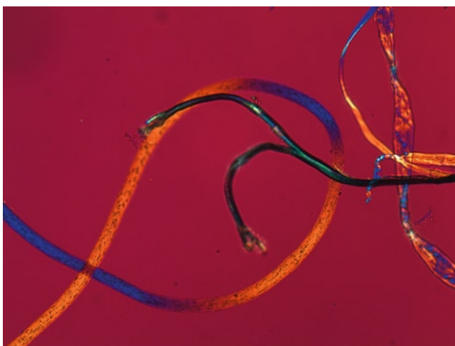
Fig. 10.4 Fibers from dust sample by polarized light microscopy. This image shows three types of fibers. The fiber on the left , with the particles on the surface, is delustered nylon whereas the one on the right in the twisted orientation is cellulose. These two fiber types are relatively easy to identify by morphology. The central fiber is less common and further tests are necessary to develop an initial hypothesis (image size = 700 \times 520 \mu\text{m} )
