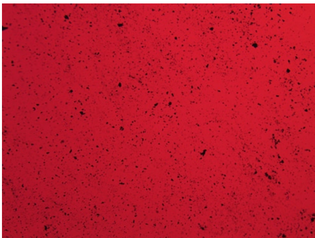
Fig. 10.9 Polarized light photomicrograph of charcoal particles. The particles are opaque and do not display interference colors. The larger particles appear to be aggregates of much smaller particles (image size = 350 \times 260 \mu\text{m} )
