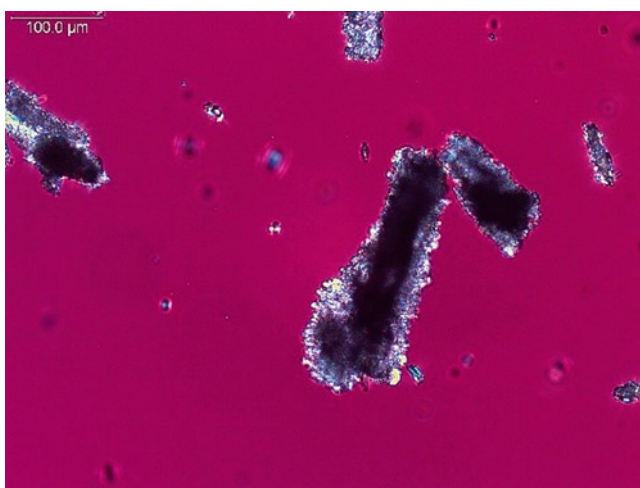
Fig. 8.7 Caffeine polarized light photomicrograph. This is a photomicrograph of caffeine as received. Note that the particle display interference colors indicating that they are crystalline. The larger particles appear to be aggregates of much smaller particles. Only one crystal habit is observed (image size = 350 \times 260 \mu\text{m} )
