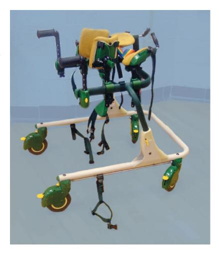
Figure R8. An important aspect of the MOVE program is the ability to get individuals into weightbearing positions, which is difficult for adult-sized adolescents. The development of mechanical lift walkers makes this process much easier for the caregivers.
