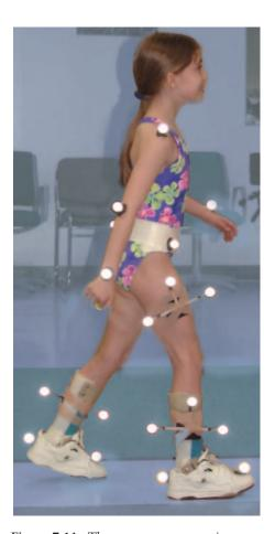
Figure 7.11. The most common gait measurement system requires that the individual being measured is instrumented with retroreflective markers that are imaged by multiple video cameras. The markers define specific anatomic body points, which the computer program uses to calculate joint motion.
