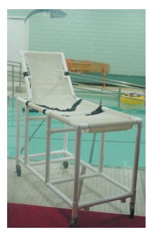
Figure R4. One problem in doing hydrotherapy for large individuals who are totally dependent for dressing and movement is finding changing rooms or tables. Low-cost solutions can easily be developed using construction and plumbing supplies. A volunteer for the school constructed this changing table.
