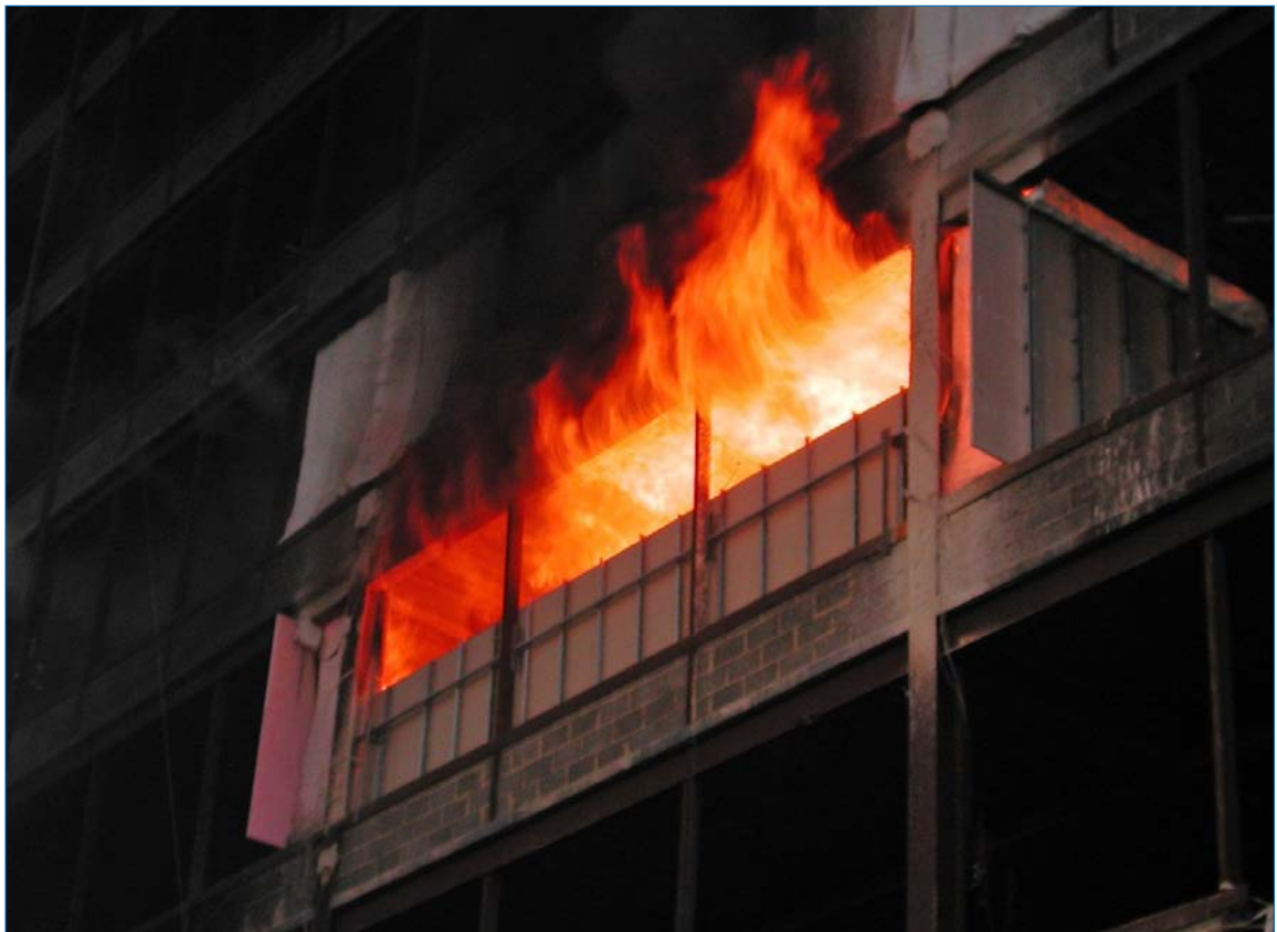
Figure 3.10 Flame behaviour through external openings © Building Research Establishment Ltd
