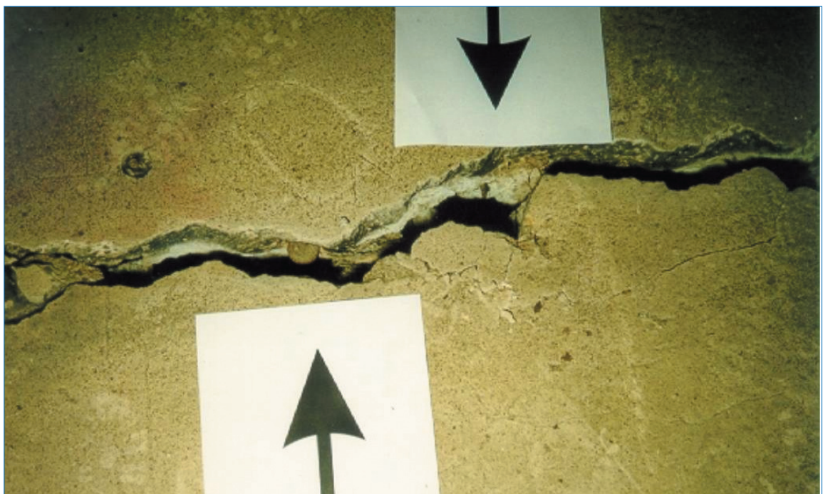
Figure 5.4 Reinforcement fracture following large scale tests 46
