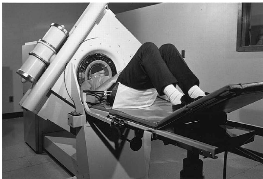
Figure 2-3. Original head CT scanner from EMI (installed at Mayo Clinic, Rochester, Minn.). Image courtesy of the RSNA.
