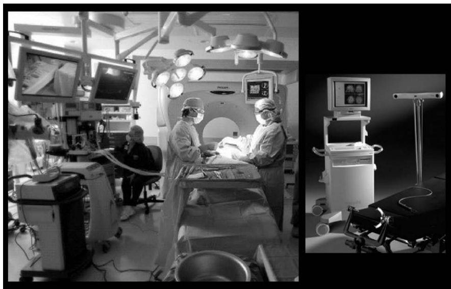
Figure 10-8. Left: Intra-operative CT (Philips Brilliance 16) at Celebration Health Florida Hospital in collaboration with Drs. Gary Onik and Joseph Redan. Right: The Philips EasyGuide, an early surgical navigation system consisting of a computer, a monitor, an optical position measurement device, and special surgical instruments.
