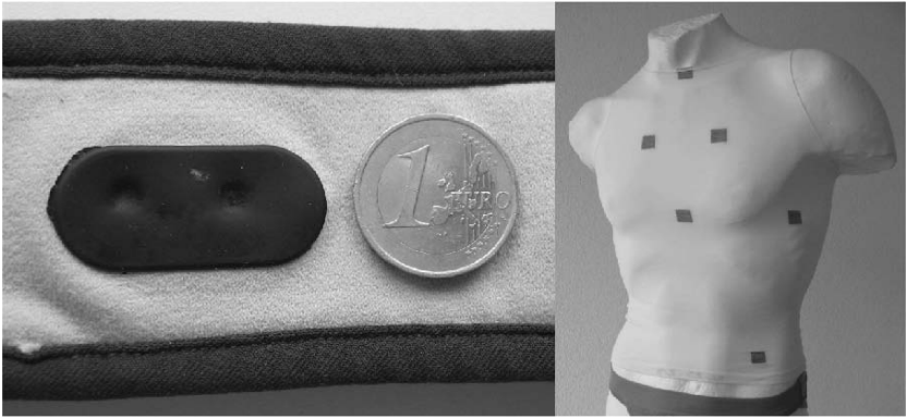
Figure 28-2. Dry electrode made of conductive rubber and integrated into a garment with shielded cable (left), textile electrodes in a garment for unobtrusive sensing of ECG (right), developed in MyHeart (European project IST-2002-507816).
