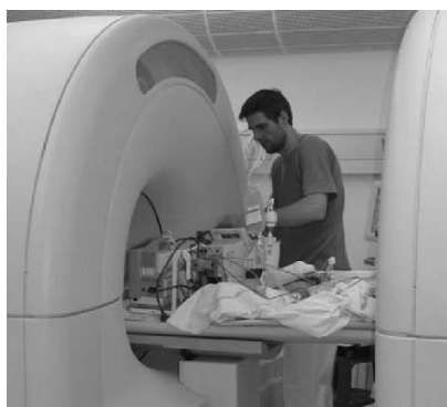
Figure 8-7. A patient under anesthesia is being scanned on Gemini™ PET/CT: the gantry is separated to allow access to the anesthetist and his equipment (Picture courtesy of I. Kastrup, Herlev Hospital, Copenhagen).
