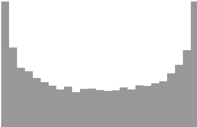
Fig. 5.3. Histogram representing the approximate probability distribution of the iterates of the logistic map f_4 : n \mapsto 4n(1 - n) . The histogram has been obtained from 75,000 iterates distributed in 25 bins
