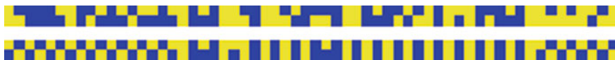
Fig. 6.36. Car traffic on a two-lane one-way road for a car density exactly equal to 0.5 on a 60-site lattice. The top figure represents the initial configuration and the bottom one the configuration after 120 iterations
