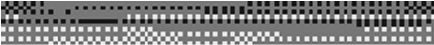
Fig. 6.5. Multilane bidirectional pedestrian traffic. Lattice length: 100; lattice width: 10; number of pedestrians: 150 moving to the left ( light gray cells ) and 150 to the right ( black cells ); number of iterations: 200. Empty cells are gray
