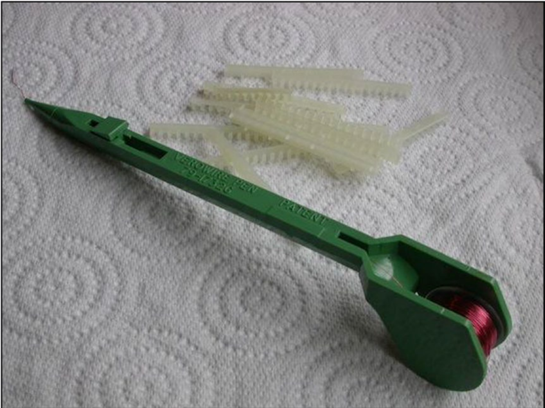
Figure 1-15. The Vero wiring pen and combs
