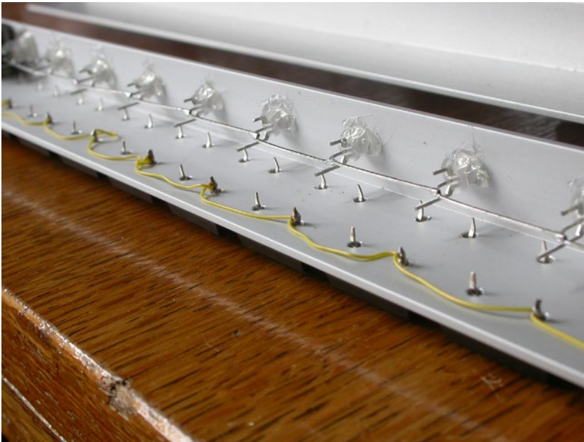
Figure 7-15. Switches and LEDs beginning to be wired up in the neck
