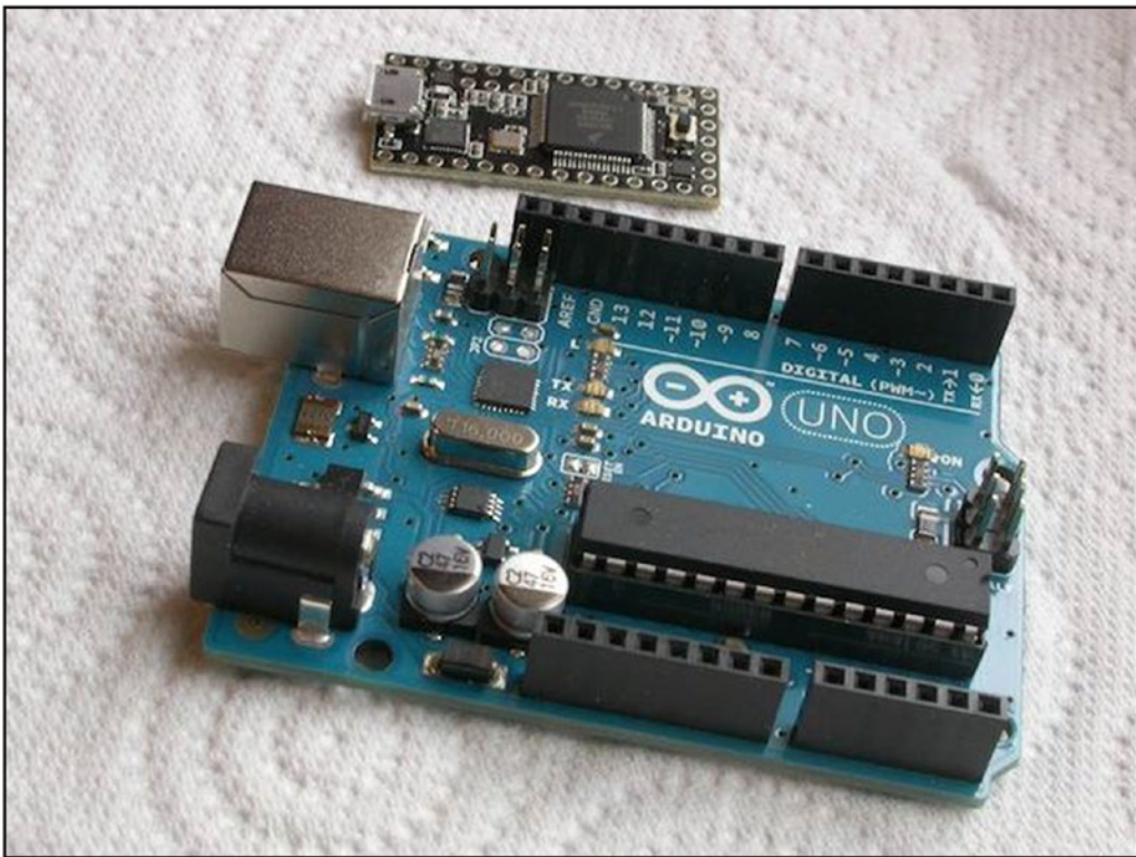
Figure 1-4. Arduino Uno and the Teensy 3.0 from PJRC
