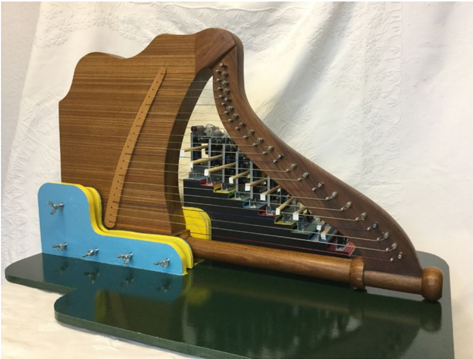
Figure 6-1. The MIDI-controlled Harp Player
