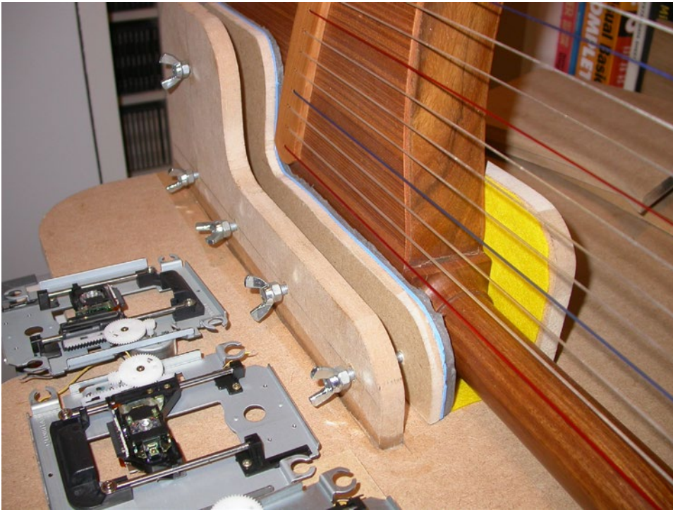
Figure 6-3. The harp's clamping arrangement
