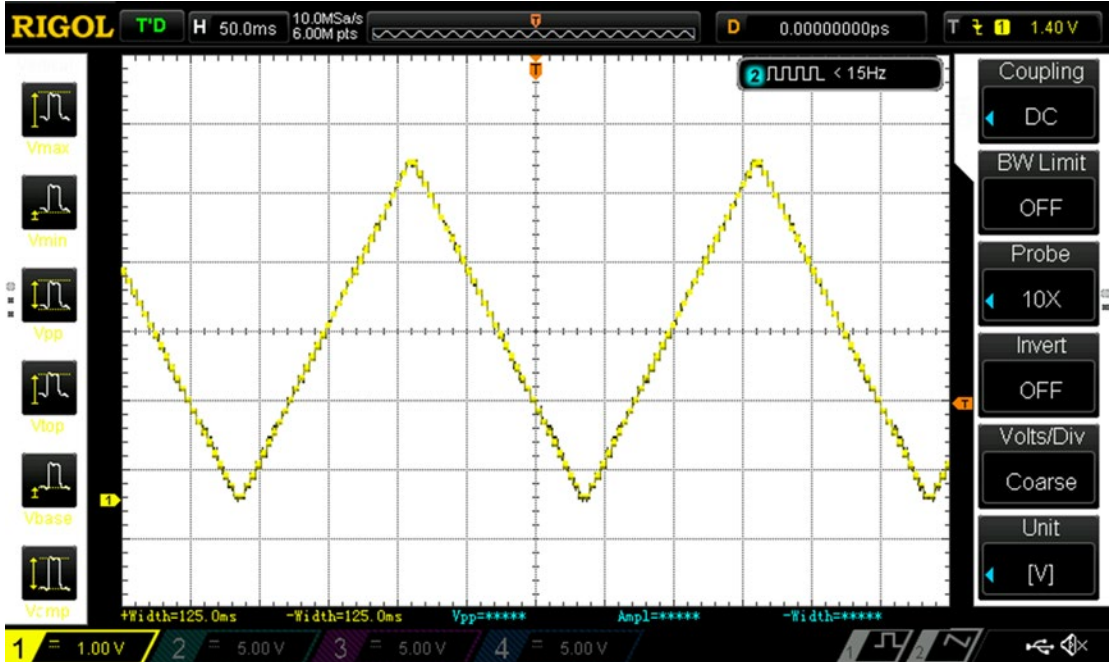
Figure 12-9. Triangle wave output
