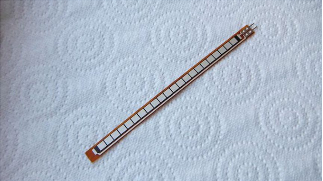
Figure 5-7. A flex sensitive resistor
