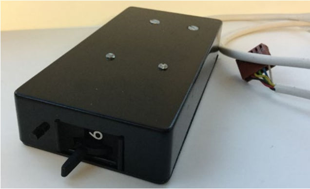
Figure 15-14. An extended hex switch
