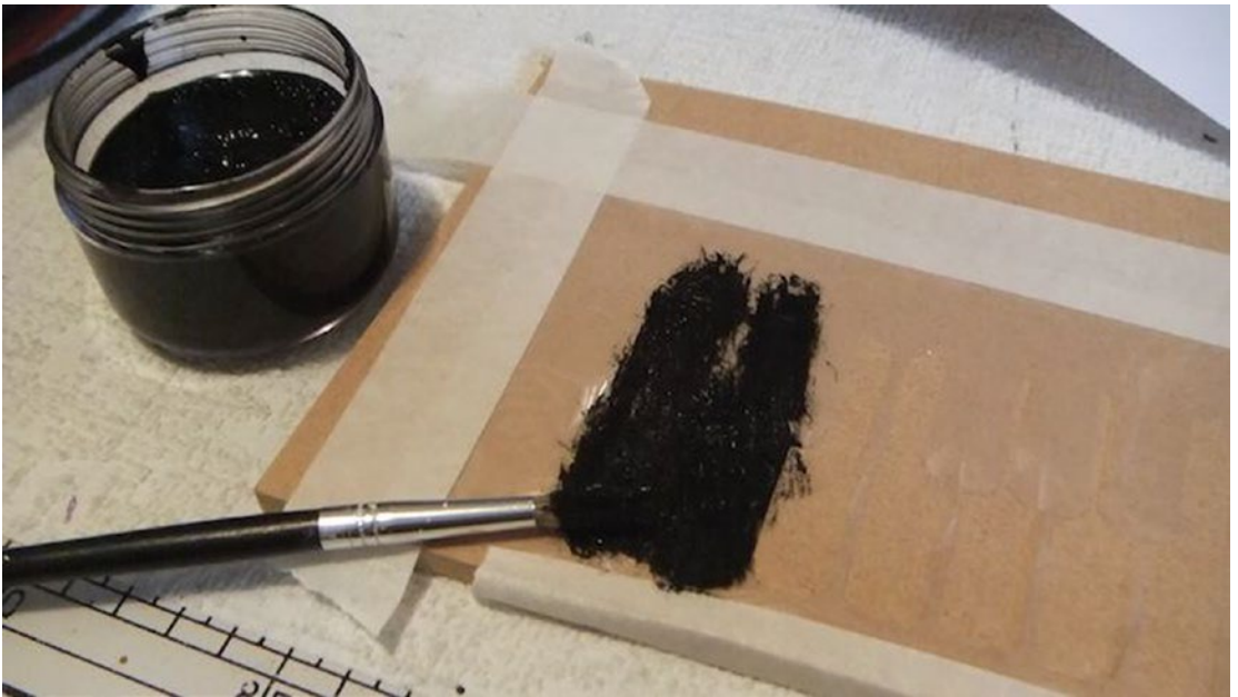
Figure 5-16. Painting through the stencil
