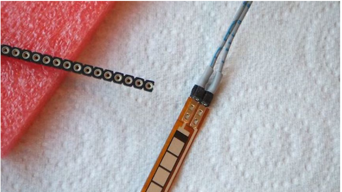
Figure 5-8. A flex sensor with socket
