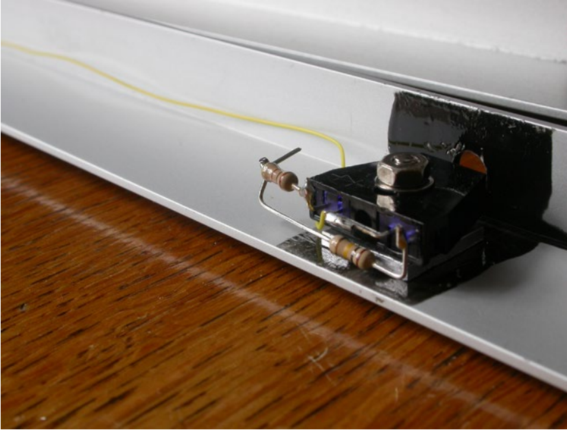
Figure 7-16. The optical reflective switch
