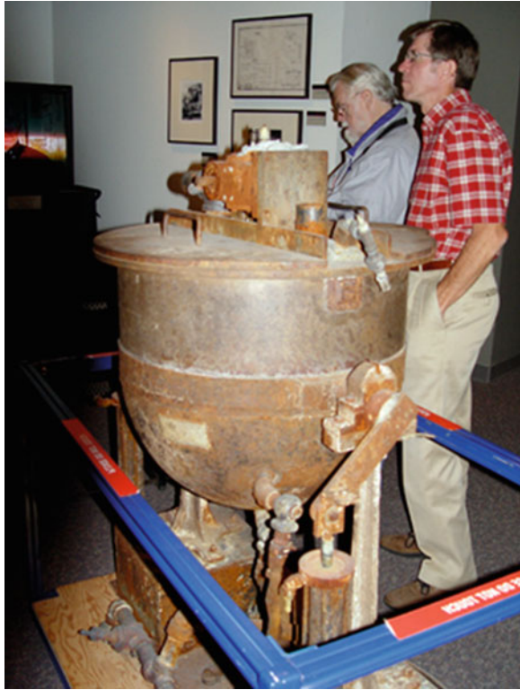
Fig. 7.23 An original implosion-lens casting machine on display at National Museum of Nuclear Science and History in Albuquerque, NM. Photo by author
