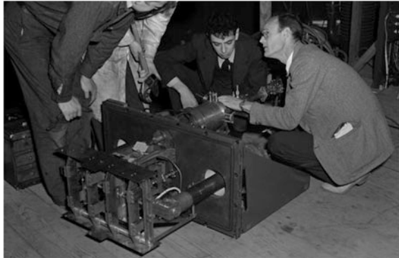
Fig. 5.16 Frank Oppenheimer ( dark hair, center ) and Robert Thornton ( right ) examine a 4-source Alpha-calutron ion emitter. Source http://commons.wikimedia.org/wiki/File:Calutron_emitter.jpg
