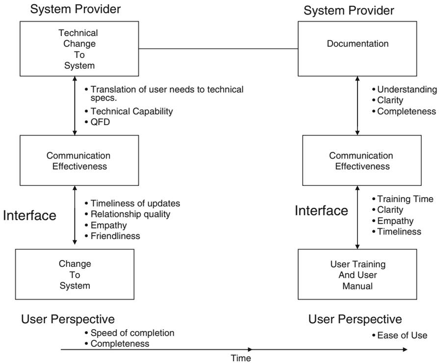
Fig. 16.4 Communicating technical changes to system
