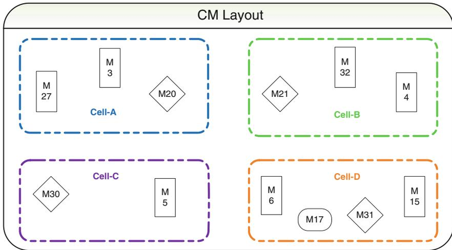
**Fig. 17.2** Machine allocation in cellular layout
