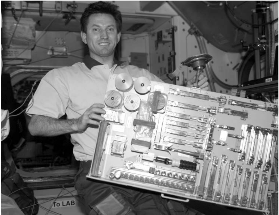
Cosmonaut Sergei Treshchev, ISS-5 flight engineer, holds a special pallet containing various tools used for orbital repairs and DIY aboard the station
