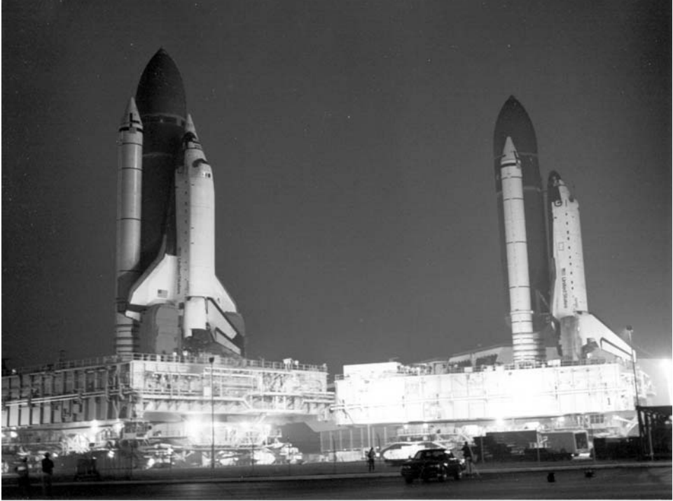
Ships that pass in the night. Columbia (left) is rolled past Atlantis (right) on its way to Pad 39A on 9 August 1990. Atlantis was parked in front of the VAB following its rollback from Pad A for repairs to its LH lines
