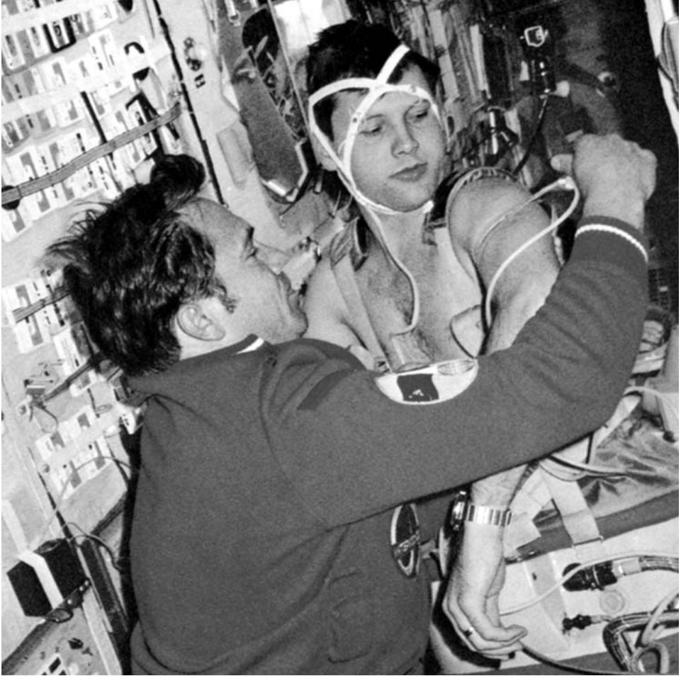
Prunariu (right) wears the Chibis lower body negative pressure garment aboard Salyut 6, assisted by Popov
