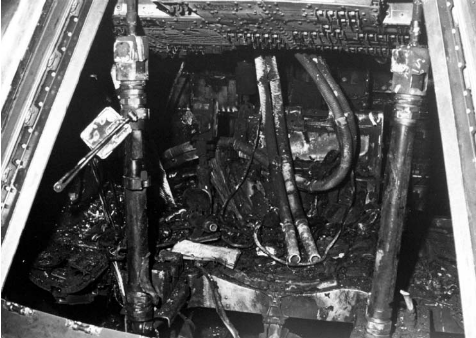
The charred inside of Apollo 204 CSM-012 following the pad fire which claimed the lives of Apollo 1 crew Grissom, White and Chaffee
