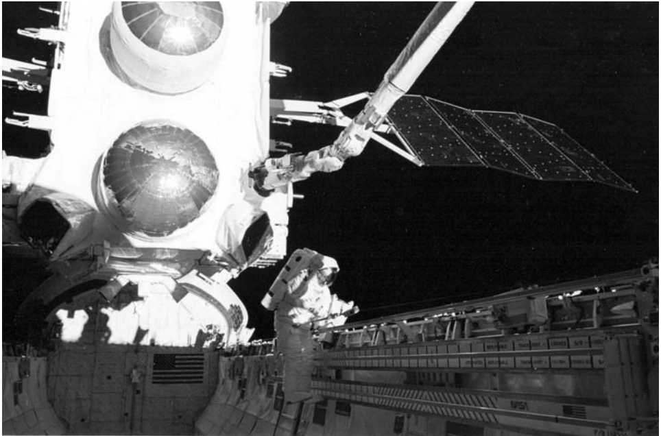
Still in the grasp of the RMS the Compton Gamma Ray Observatory is held above Jay Apt during the successful 7 April EVA to free its high-gain antenna
