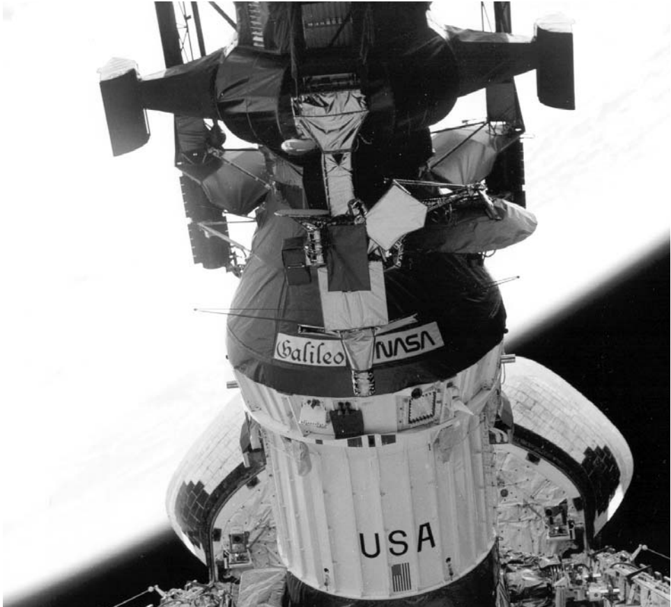
Galileo is deployed from Atlantis atop its IUS to start its long journey to Jupiter
