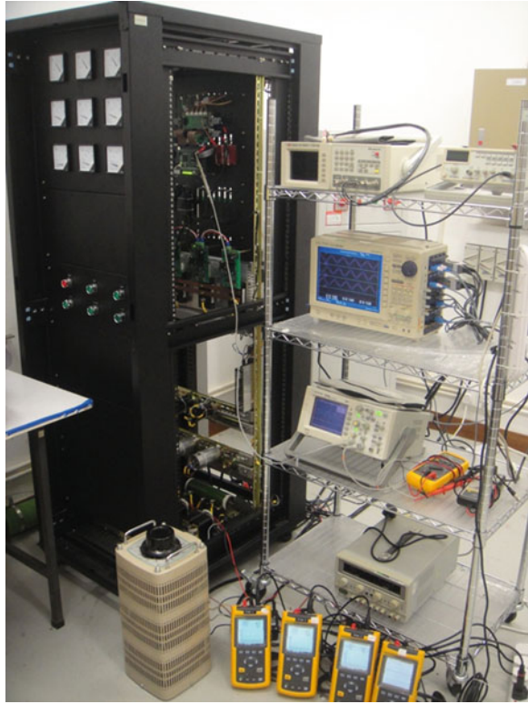
Fig. 6.9 The 220 V, 10 kVA HAPF experimental prototype testing environment
