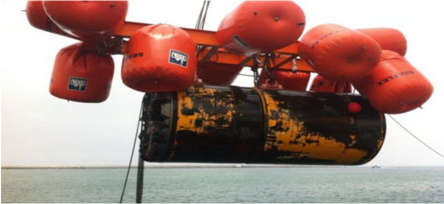
Fig. 6.5 Recovery of tunnelling machine via airbags and lifting by crane in harbor
