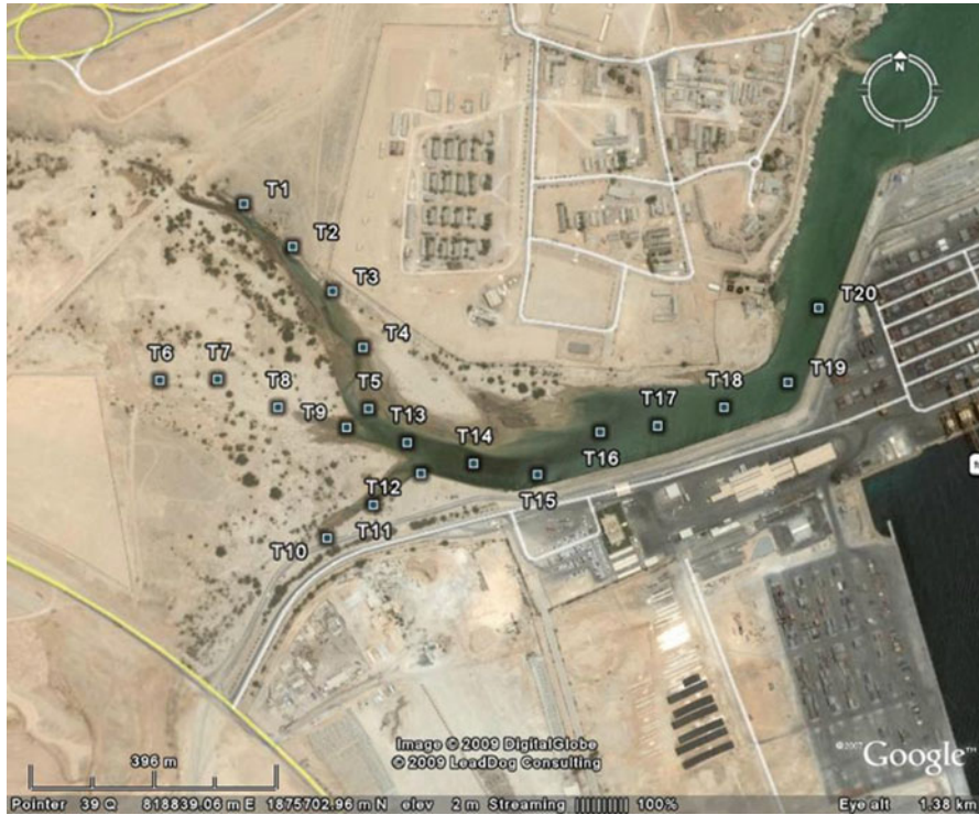
Fig. 19.1 Lagoon area adjacent to Port Salah. Transect locations for bathymetric survey are also shown and the outlet is located close to T6 (Google Earth)
