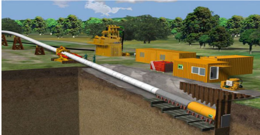
Fig. 6.14 Direct Pipe® view on shaft with Pipe Thruster
