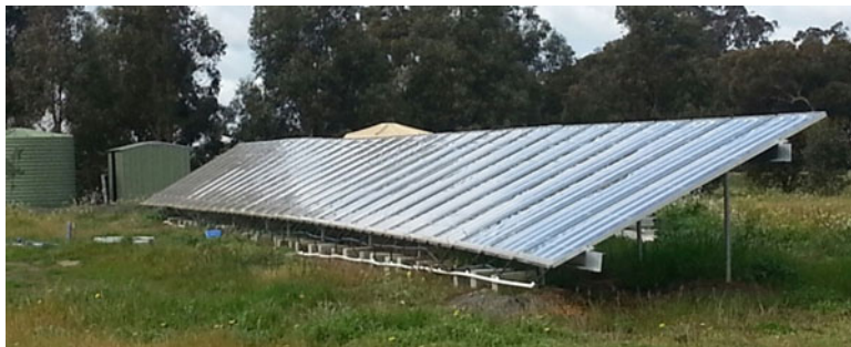
Fig. 12.10 Australian made Carocell wick distillation units at Kendenup near Albany in Western Australia
