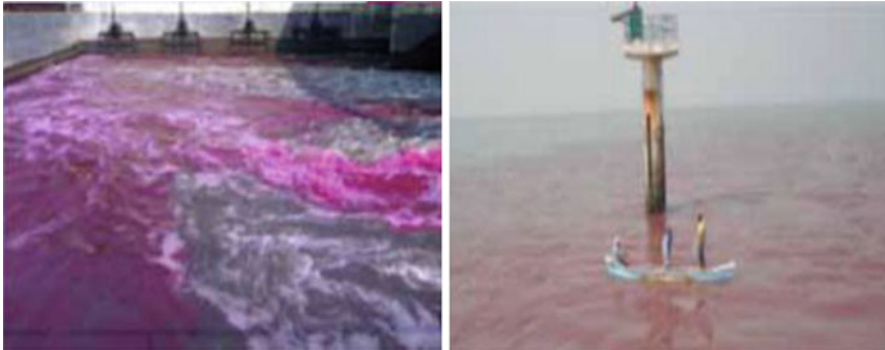
Fig. 21.6 Rhodamine application after grit chamber and near diffuser pole
