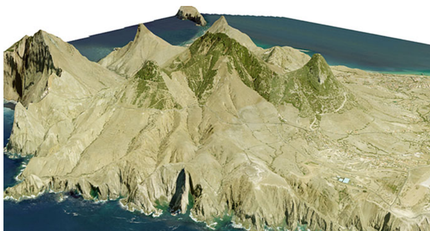
Fig. 4.41 Perspective representation of a DTM with draped orthoimage (Porto Santo Island)
