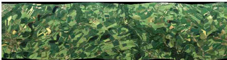
Fig. 4.7 A RGB composite image acquired with an ADS camera and corrected from attitude variation (Leica Geosystems)
