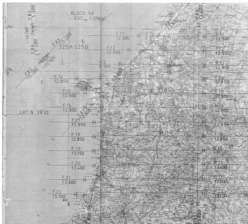
Fig. 4.18 Flying map showing strips, start and end exposure points and flying height in feet
