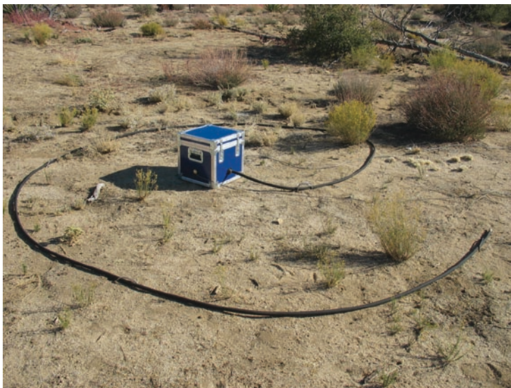
Fig. 5.14 Photo of a spiraling-outward microporous hose connected to a microbarometer at Piñon Flat Observatory
