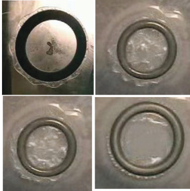
Fig. 12.12 Surface waves in a two-dimensional shallow circular layer of liquid nitrogen around a rigid core. Modes with l = 12\text{--}30 and amplitude in the range 1–5 mm can be measured, depending on the depth of the layer. The waves travel with a circular speed of 20\text{--}40\text{ cm s}^{-1} . In the figure the core has a diameter of 3 cm
