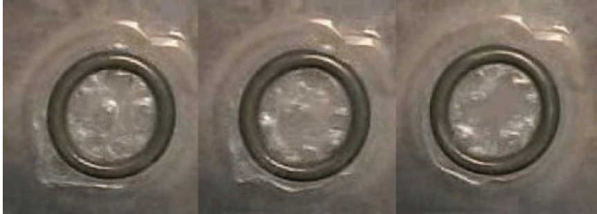
Fig. 12.14 Traveling and decaying of cnoidal waves on the external surface taken at three different moments of time
