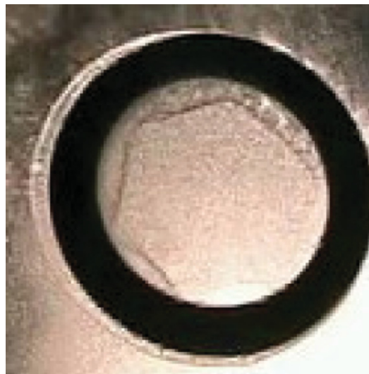
Fig. 12.13 Internal surface waves in a liquid nitrogen shell, upper bounded by a rigid core. In the figure one can see a clean l = 6 mode, with amplitude 2.5 mm, traveling with a speed of 12\text{ cm s}^{-1} . The wave was stable for about 4 s, and broke up only because of evaporation and volume loss
