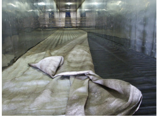
Plate 6.2 Interior of a composting tunnel. Compost is filled in a layer about 2.5 m deep on top of a mat. Air is blown in underneath the compost to allow an aerobic composting process.
