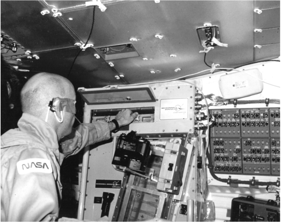
Musgrave monitors the Continuous Flow Electrophoresis System (CFES) loaded aboard the mid-deck of Challenger during STS-6
