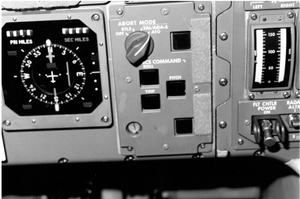
The Abort-to-Orbit control is clearly displayed in this photo of the flight deck controls of Challenger after the STS 51-F launch suffered the loss of a main engine.
