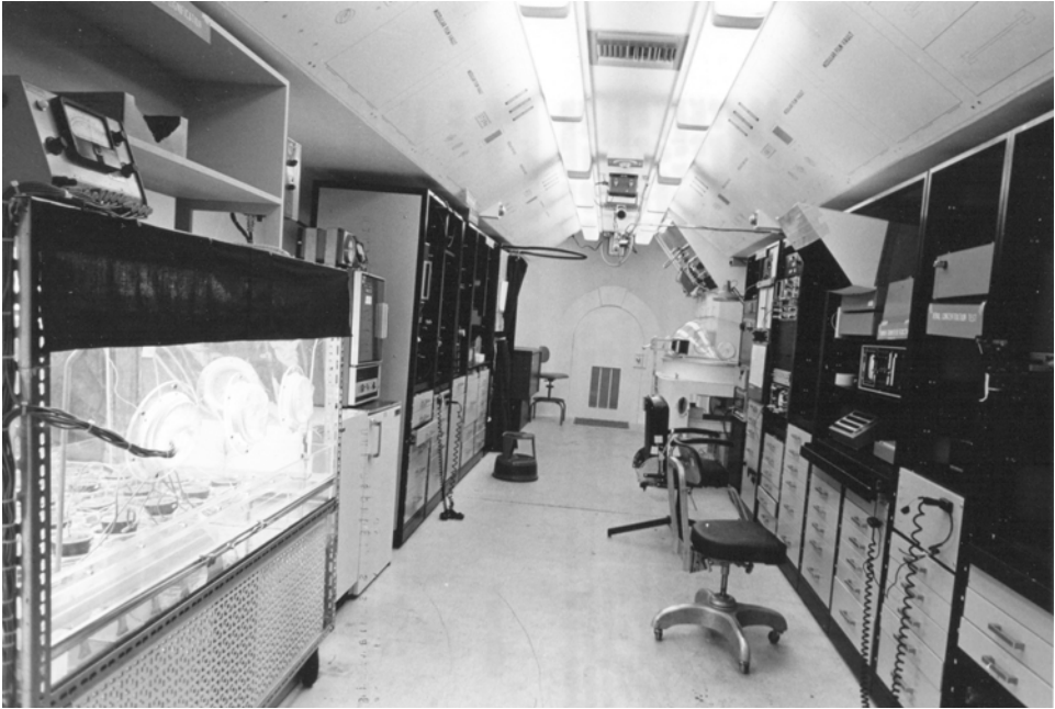
The interior of the October 1974 SMS module showing the laboratory-like racks to simulate Spacelab science racks.
