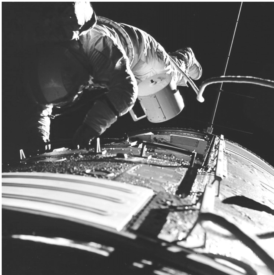
Command Module pilot Ron Evans is photographed retrieving film canisters during his trans-Earth-coast EVA to the rear of the spacecraft.
