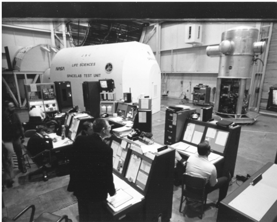
The SMD mock-up configured for the second test, with the cosmic ray experiment located at right rear simulating a Shuttle pallet payload.
