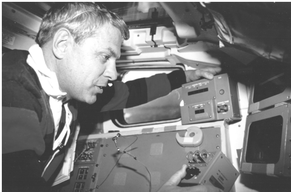
Parker uses a manual pointing controller for the Astro-1 mission's Instrument Pointing System from the aft flight deck of Columbia during the STS-35 mission.
