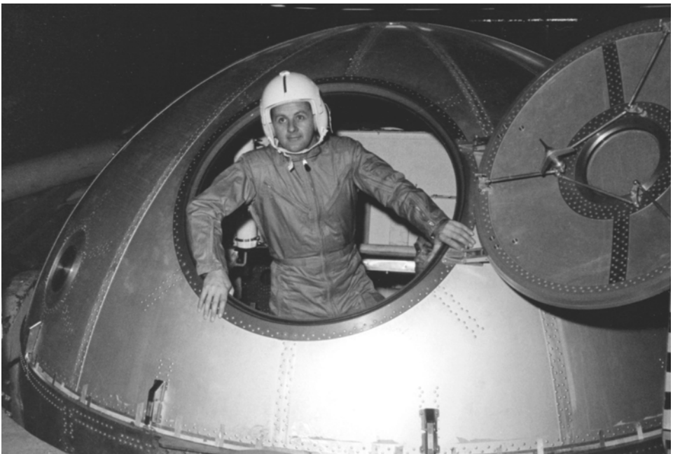
In March 1968, Phil Chapman stands in the centrifuge gondola of the Manned Spacecraft Center's Flight Acceleration Facility.
