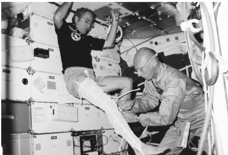
Thornton measures the leg volume of Dick Truly using a stocking plethysmograph. The test was part of the ongoing studies into in-flight fluid changes, part of Thornton's DSO programme.
