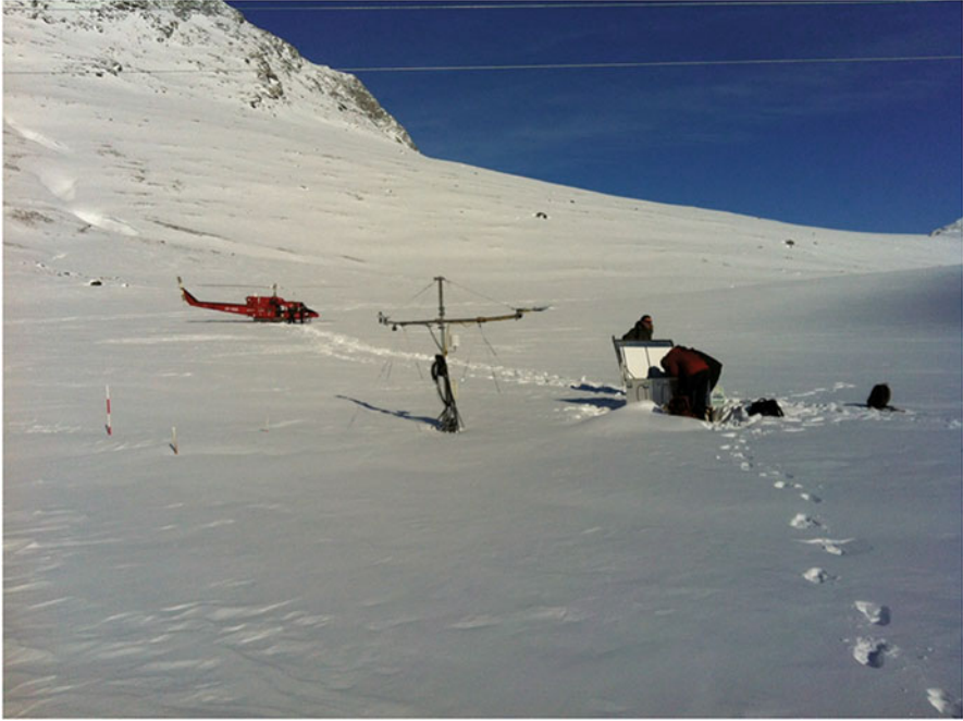
Fig. 20.6 Downloading and checking equipment at an INTERACT site (Nuuk, west Greenland) to record exchanges of energy and water between the ground surface and lower atmosphere (Photo: T. R. Christensen)
