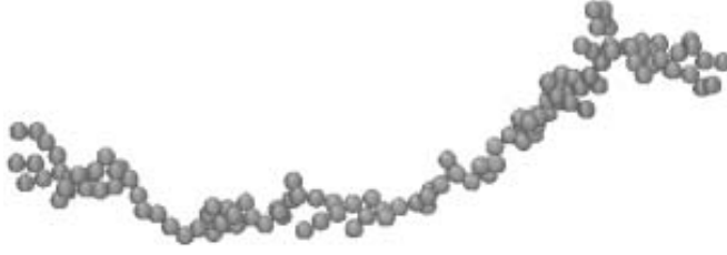
Fig. 7.12. Figure of cluster cluster aggregate with parameters diameter of primary particle d = 30 nm, fractal dimension D_f = 1.3 , radius of gyration r_g = 4.5462 \mu\text{m} , 130 primary spheres.
