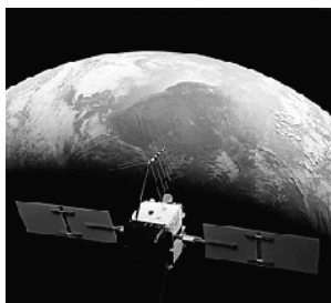
Fig. 7.9. Satellite of the GPS Navstar system. There are 24 of them orbiting around the Earth.
