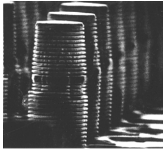
Fig. 1.1. Forest of microlasers, each of which is a pile of pancakes of alternating slices of GaAs and GaAl semiconductors. The diameter of each element is 0.5 micrometers, the height is 7 micrometers.
