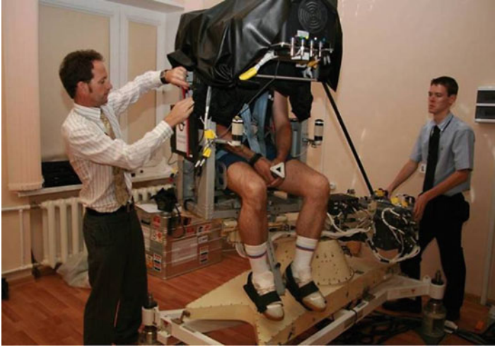
Fig. 2.21 Roscosmos cosmonaut Yuri Malenchenko seated on the visual and vestibular investigation system in star city in Moscow, undergoing a final check before centrifugation (Source: GCTC Moscow)
