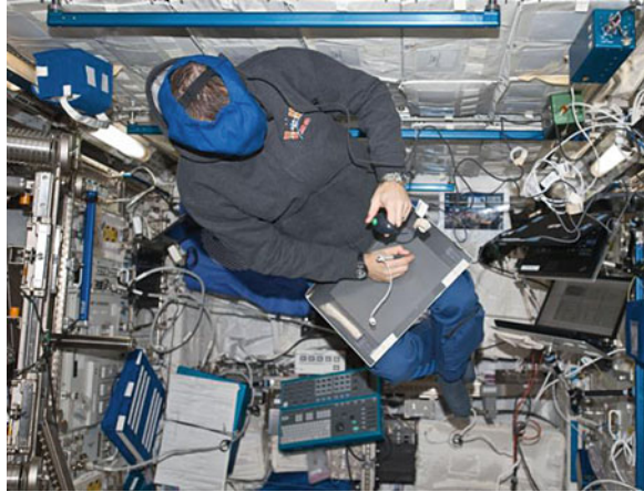
Fig. 3.36 ESA Astronaut Paolo Nespoli performing the 3D-SPACE experiment on board the ISS. He interacts with 3D views presented in a head-mounted display (the hood is used to block any external light that could give orientation cues). The digitizing tablet is used for neuropsychological testing of writing and drawing geometrical figures in absence of visual feedback (Source: courtesy of ESA)
