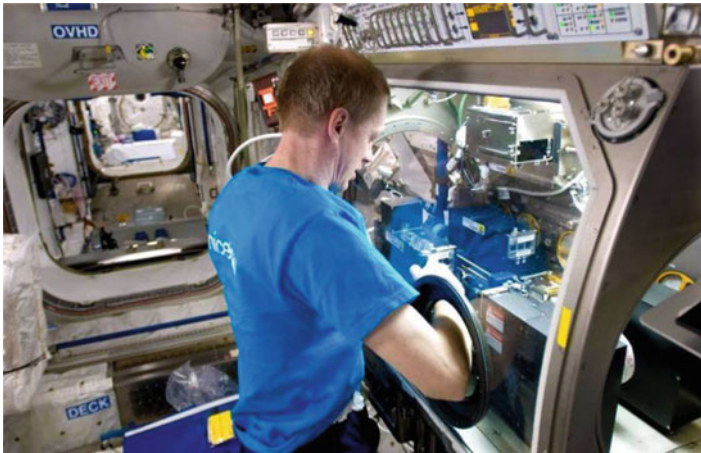
Fig. 2.7 ESA astronaut Frank De Winne during installation of the selectable optical diagnostic instrument hardware into the Microgravity Science Glovebox in 2009 (Source: NASA)
