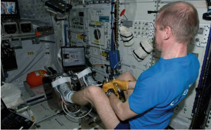
Fig. 2.5 ESA astronaut and ISS Expedition 21 Commander Frank De Winne checking out the ESA Flywheel Exercise Device, with the in the Columbus laboratory of the International Space Station (Source: NASA)
