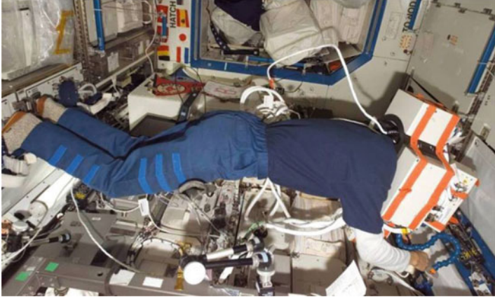
Fig. 2.9 NASA astronaut and Expeditions 14 and 15 Flight Engineer, Sunita Williams, wears the anomalous long term effects in astronauts' central nervous system (ALTEA) experiment helmet while conducting the experiment in the US laboratory (Source: NASA)
