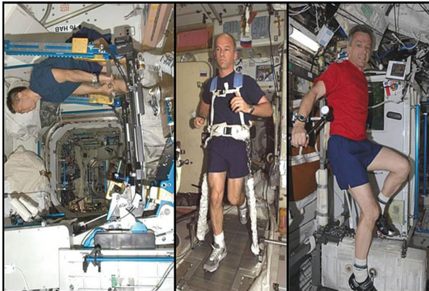
Fig. 3.39 The three exercisers used on the ISS, from left to right aRED, TVIS & CEVIS (Source: NASA)
