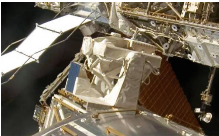
Fig. 2.11 The solar payload facility pictured on the Columbus laboratory during the STS-124 mission (Source: NASA)
