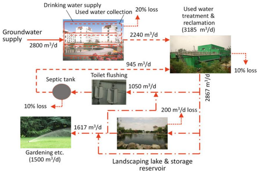
Fig. 4.5 Configuration of the on campus water system. Photo images and graph by Wang XC
