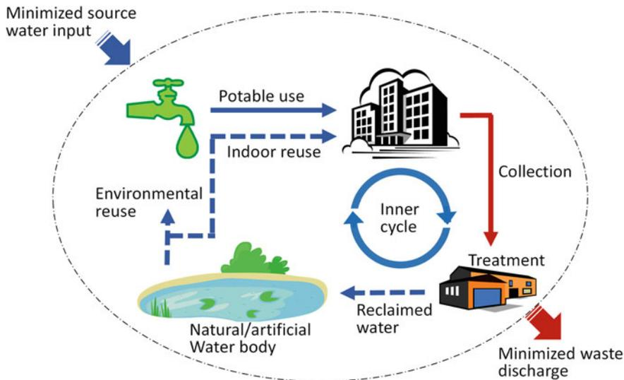
**Fig. 2.8** A decentralized water system as an independent water cycle (graph by Wang XC)
