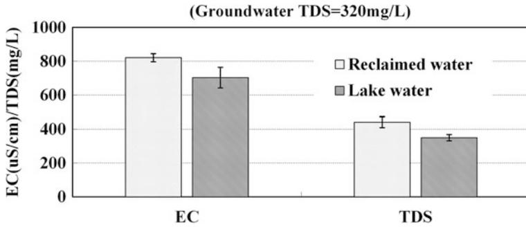
**Fig. 4.11** Comparison of the reclaimed water and lake water for salt contents in terms of TDS and EC. *Source* Unpublished data of the authors, graph by Wang XC
