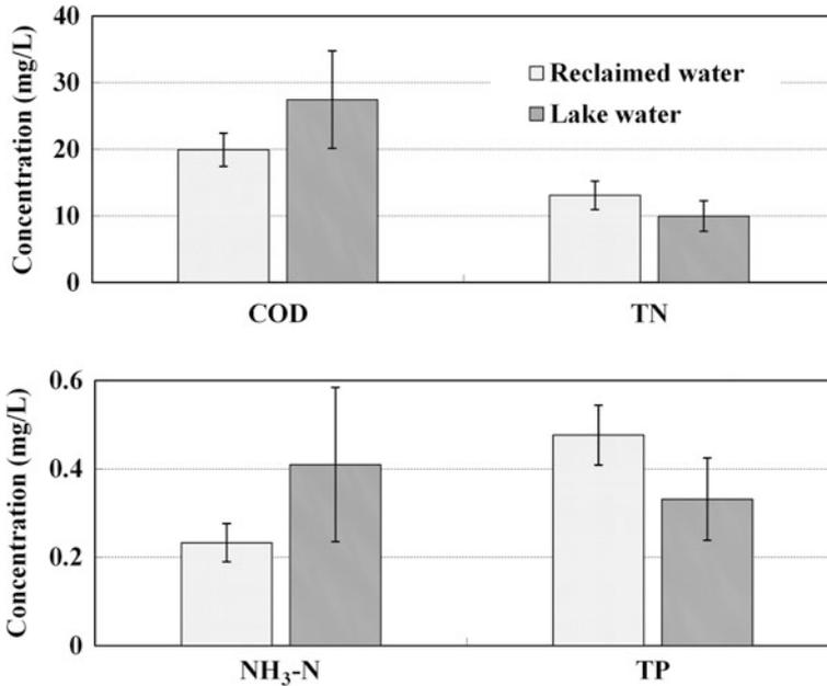
**Fig. 4.10** Comparison of the reclaimed water and lake water for conventional water quality parameters. *Source* Unpublished data of the authors, graph by Wang XC
