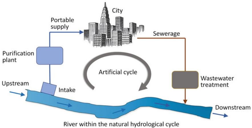
**Fig. 2.6** Conventional urban water system as an artificial water cycle attached to the natural hydrological cycle (graph by Wang XC)
