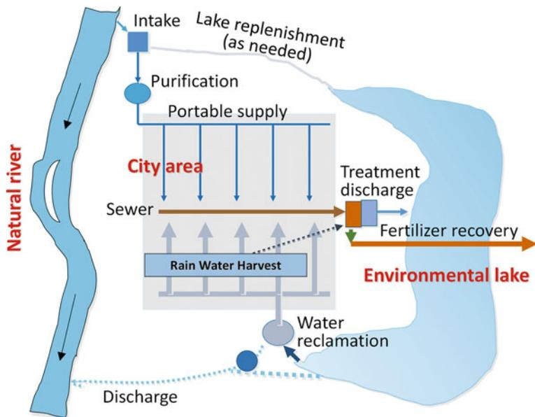
**Fig. 2.7** A water district integrating water supply, wastewater treatment and reuse, and urban water environment in one framework. Adapted from Tambo et al. (2012) by permission from Journal of Water Sustainability, copyright 2012
