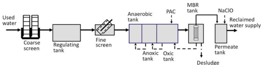
**Fig. 4.7** Schematic diagram of the used-water treatment and reclamation process. Full capacity of treatment as 4,000 m<sup>3</sup>/d, graph by Wang XC
