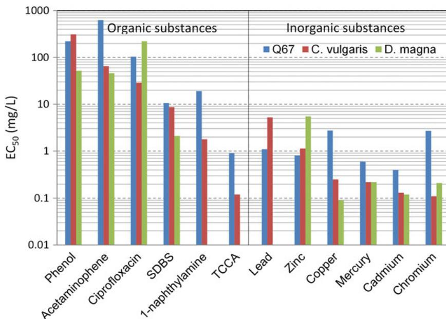
**Fig. 3.4** Comparison of toxicities measured using bacteria (Q67), alga (*C. vulgaris*), and daphnia (*D. magna*). Source Unpublished data of the authors, graph by Ma XY
