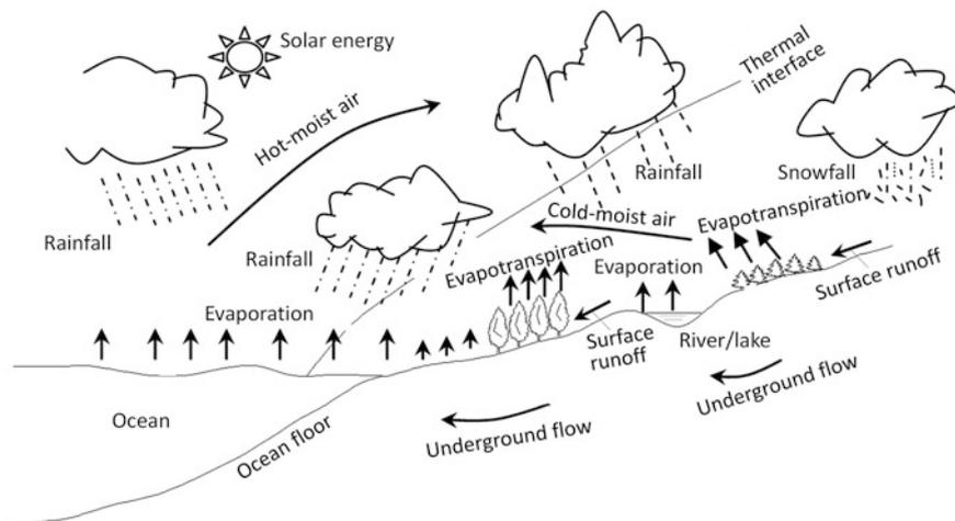
Fig. 2.2 Global hydrologic cycle (graph by Wang XC)
