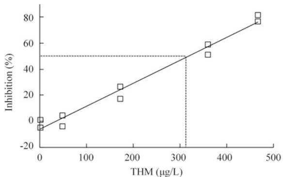
indicating that DPB formation does contribute to an increase in ecotoxicity after disinfection. An understanding of the relationship between THM formation and its potential toxicity can provide the basis for reconsidering the disinfection process for reclaimed water quality control.
