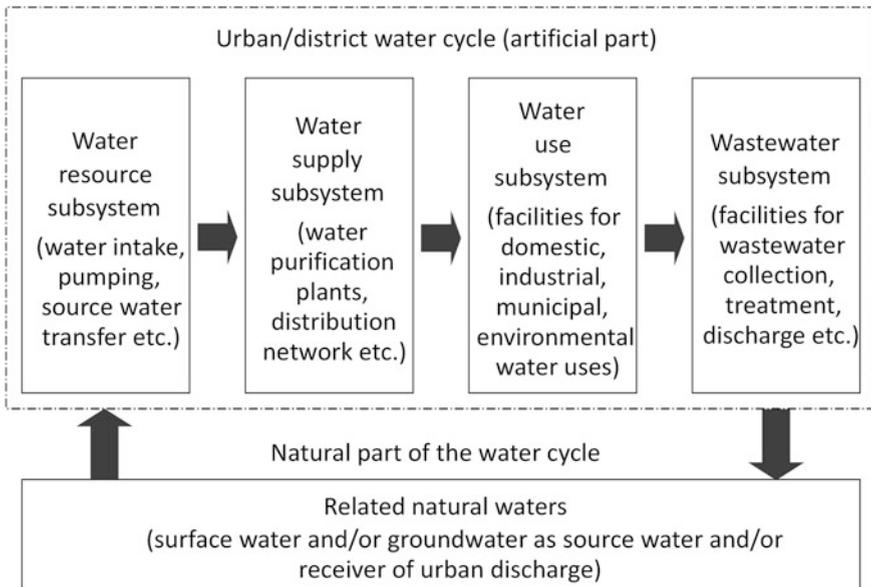
**Fig. 2.9** Composition of an urban/district water system and the formation of a water cycle consisting of the artificial and natural parts (graph by Luo L)
