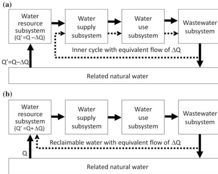
**Fig. 2.10** Models of wastewater reuse for **a** water saving, and **b** water resource enlargement.  $\Delta Q$  is the flow rate of the reclaimable water (graph by Wang XC and Luo L)
