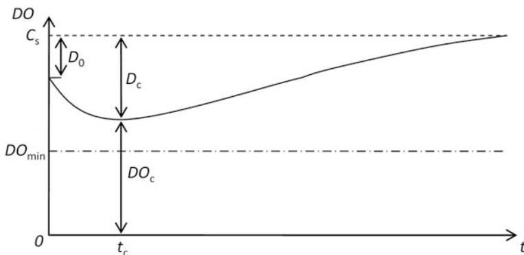
**Fig. 2.5** Oxygen sag curve obtained as the solution of Streeter and Phelps equations.  $DO_{\min}$  is the standardized minimum dissolved oxygen concentration;  $DO_c$  is the dissolved oxygen concentration at the bottom of the sag curve corresponding to time  $t_c$ ; and  $D_0$  and  $D_c$  are initial and maximum oxygen deficits, respectively (graph by Wang XC)
