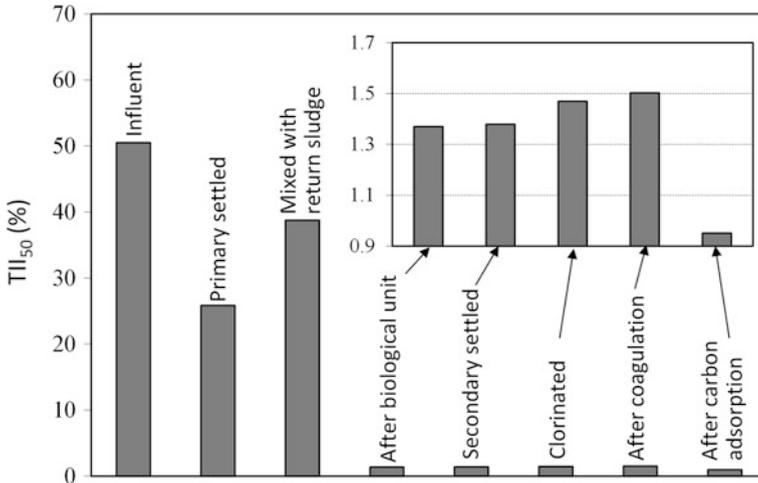
**Fig. 3.6** Variation of ecotoxicity along a wastewater treatment and reclamation process. Adapted from Ma et al. (2011), by permission from Elsevier Limited, copyright 2011
