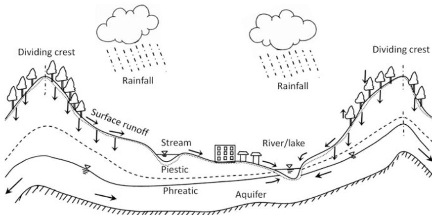
**Fig. 2.3** Surface and subsurface flows in a watershed (graph by Wang XC)
