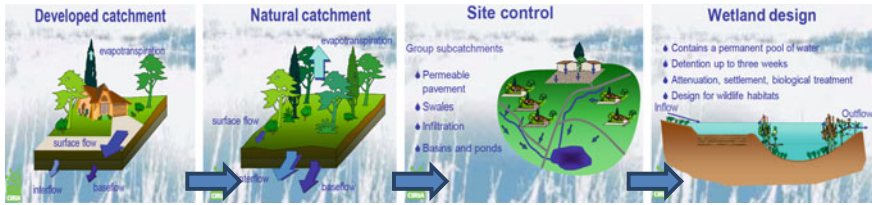
Fig. 6 From natural to developed (built) and back to natural principles in surface run-off
