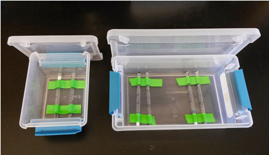
Fig. 2 A humidified chamber for ISH incubations. Serological pipettes are cut to the appropriate length and attached to the bottom surface of the Tupperware with laboratory tape. The distance between the each set of pipettes is adjusted to accommodate the width of the slide. Water soaked paper towels are placed inside the chamber to create a moist environment for incubations
