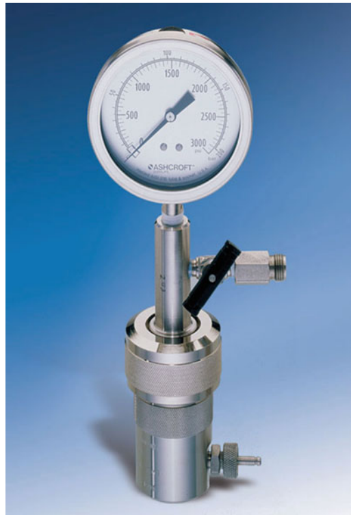
Fig. 1 A cell disruption chamber for nitrogen decavitation (Parr® Instruments). The cell suspension is placed inside the chamber, which is closed and filled with \text{N}_2 . When the suspension, still under pressure, is slowly let out through a valve at the bottom of the chamber, the cells will disrupt due to rapid decompression
