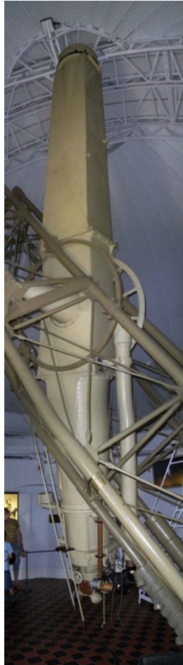
The 28-in. photovisual refractor at the old Royal Observatory, Greenwich, completed in 1893, whose giant lens was to allow the telescope to perform as an observational and photographic instrument (Credit: Peter Grego)
