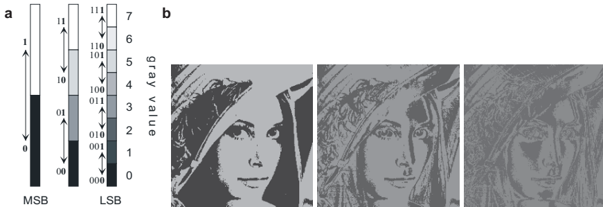
Fig. 6.3. a Contributions of single bits to overall gray levels of a 3 bit discrete amplitude representation. b Left to right: Bit planes 1 (MSB), 2 and 3 (LSB) of a 3-bit PCM signal.
