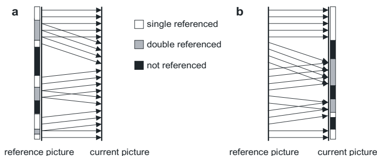
Fig. 7.5. Motion compensation using current picture (a) and reference picture (b) for the coordinate system
