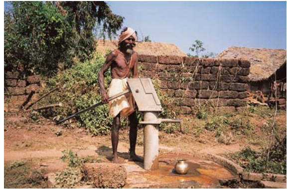
Plate 97: Shallow well – Handpump, Orissa State, India, November 1999.
