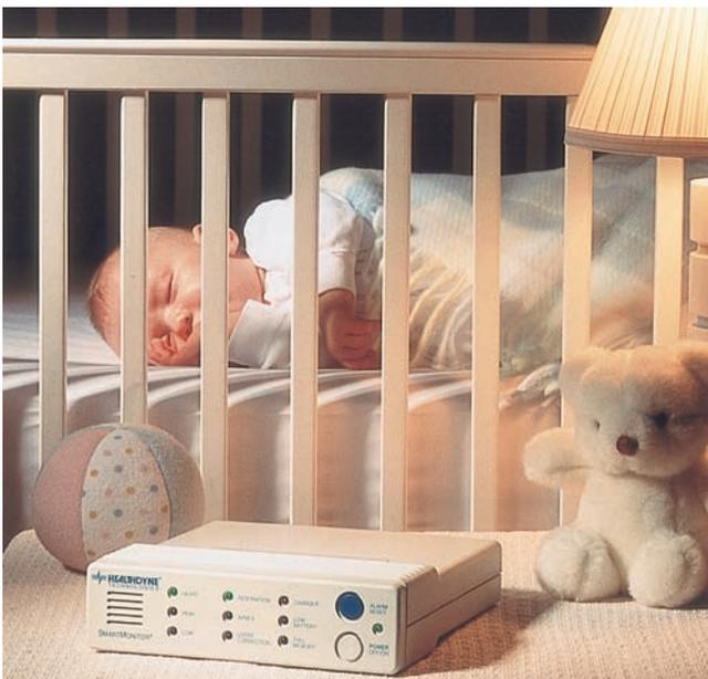
**FIGURE 26.10** An apnea monitor for home monitoring. (Photograph courtesy of Respiroics/Healthydyne Technologies, Marietta, GA.)
