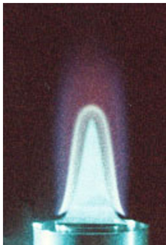
Fig. 7.13. A laser tomogram of a methane–air premixed flame at low pressure (photo from the Laboratoire d’Aérothermique du CNRS, private communication, 1985)
