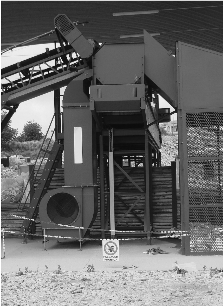
9.4 Air sifting separation arrangement within a level 1 CDW recycling plant.
