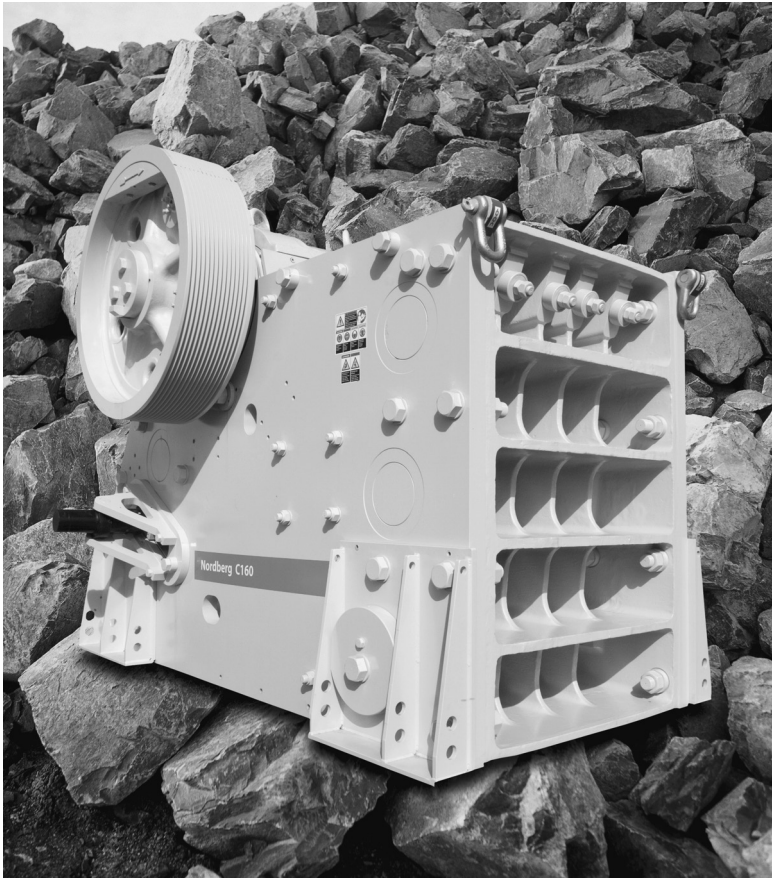
9.7 Example of a jaw crusher (Metso, 2012).
