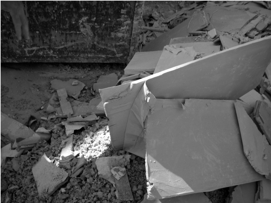
19.6 Waste gypsum board.
