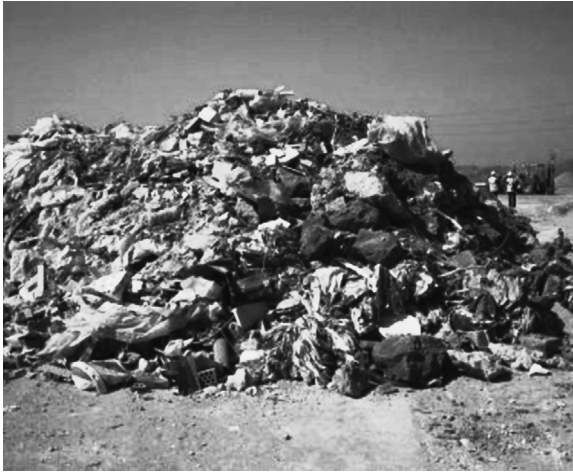
3.1 Construction waste is a heterogeneous mixture composed mainly of soil, packaging waste, debris and a low percentage of hazardous waste.
