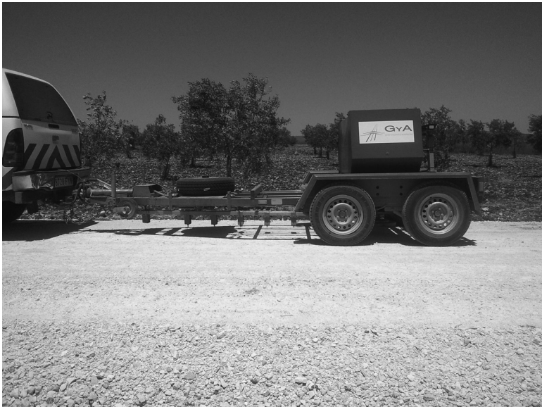
14.7 Falling weight deflectometer mounted on a trailer.
