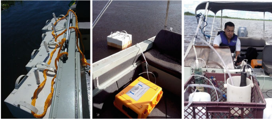
Fig. 2 Sampling technique of chamber gas fluxes with gas sampling for later GC–FID analysis (April–May 2011, picture on the left ) and in situ measurements of chamber fluxes and gas partial pressure (equilibrator) with the UGGA-LGR (March–April, 2014, pictures in the middle and to the right )
