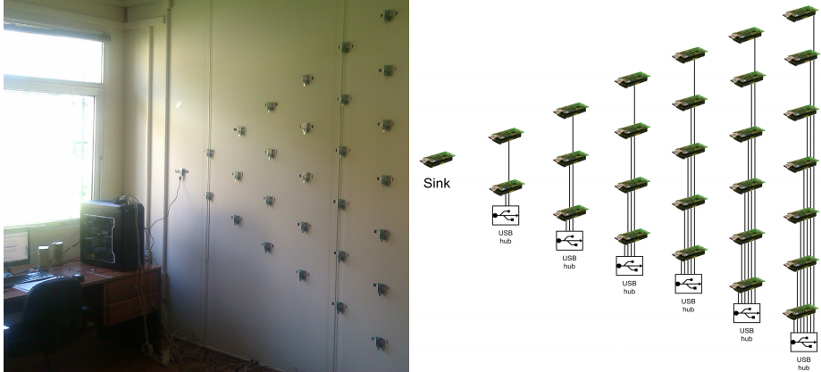
Fig. 4. The USB-wired node topology
