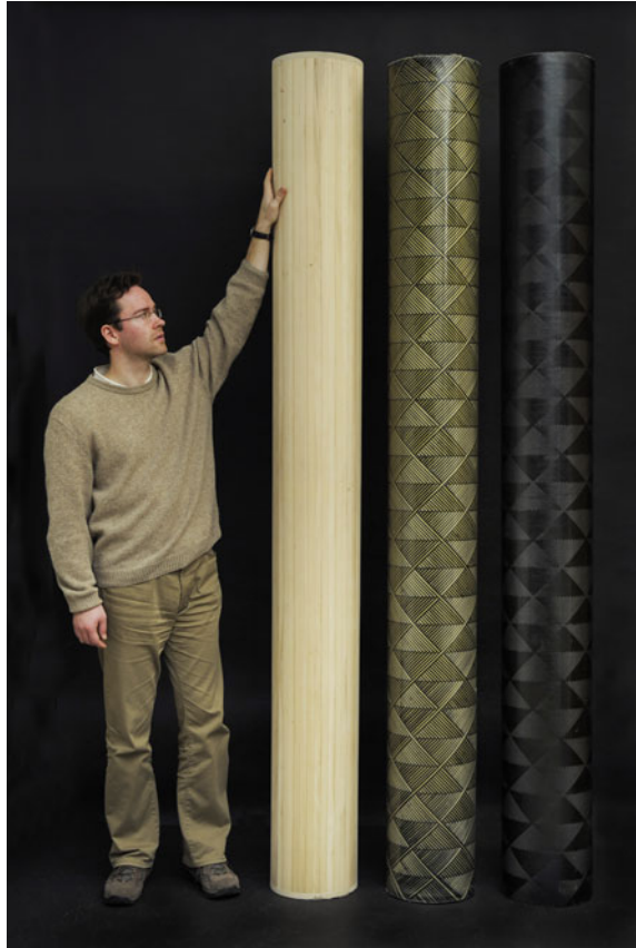
Fig. 5 Moulded tube from Norway spruce with a length of 250 cm, a diameter of 28 cm, and a thickness of the tube wall of 2 cm, fibre reinforcements: ( middle ) filament winding of aramid and carbon, ( right )
