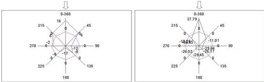
Fig. 8.18 Comparison of experimental mean pressures values ( left ) and numerical results ( right ) at the middle cross-section of the tower with turrets influencing the flow
