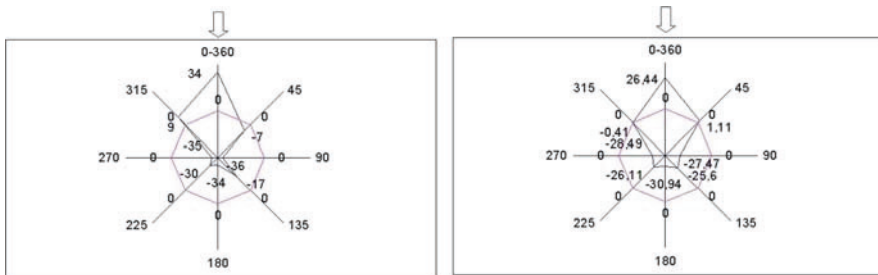
Fig. 8.17 Comparison of experimental mean pressures values ( left ) and numerical results ( right ) at the upper part cross-section of the tower with turrets
