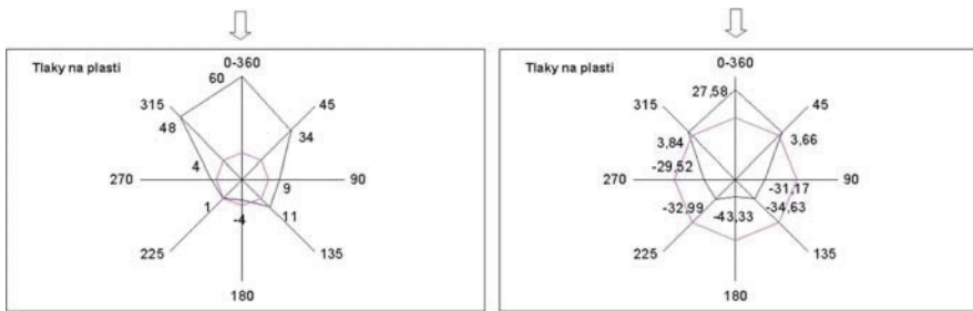
Fig. 8.16 Comparison of experimental mean pressures values ( left ) and numerical results ( right ) at the mid cross-section of the simple (turrets-free) tower
