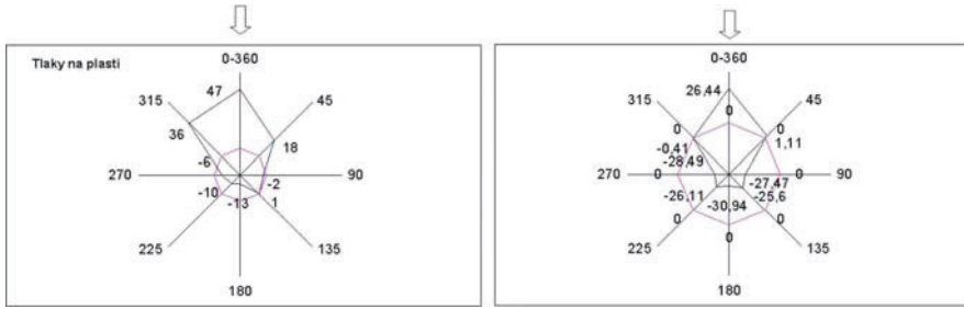
Fig. 8.15 Comparison of experimental mean pressures values ( left ) and numerical results ( right ) on the top of the simple (turrets-free) tower
