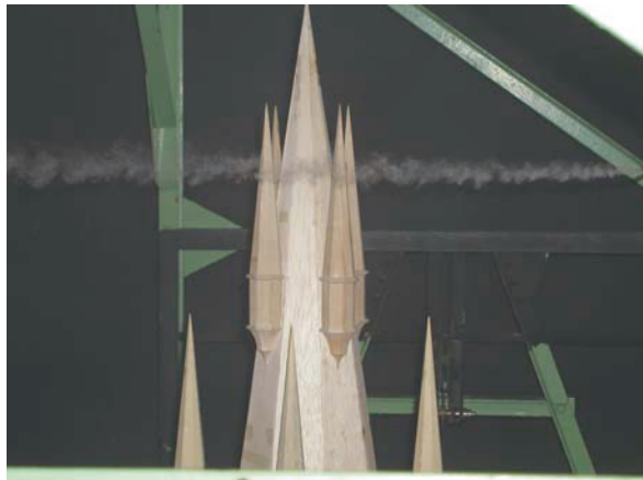
Fig. 8.19 The view of the scaled (1:25) validation model of the tower in the wind tunnel during simultaneous pressure measurement and flow visualization using smoke trailer
