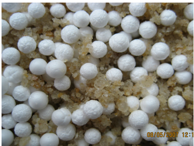
FIG. 2. Sand-EPS beads mixture.
