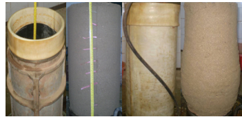
FIG. 5. Compaction degree control and sampling process.
