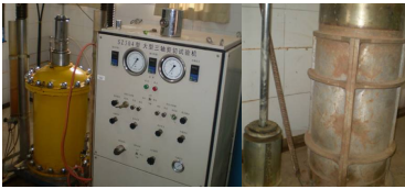
FIG.2. SZ304 triaxial test apparatus and sampling devices.
