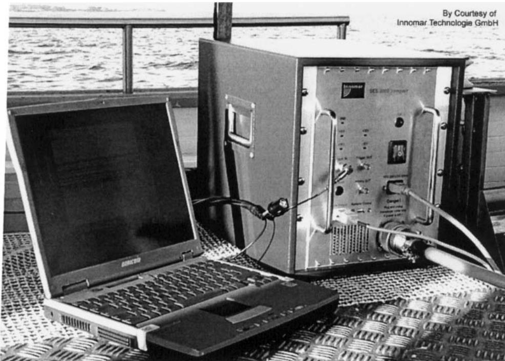
Figure 133: Laptop PC with Innomar SES 2000 Compact - parametric sub-bottom profiler
