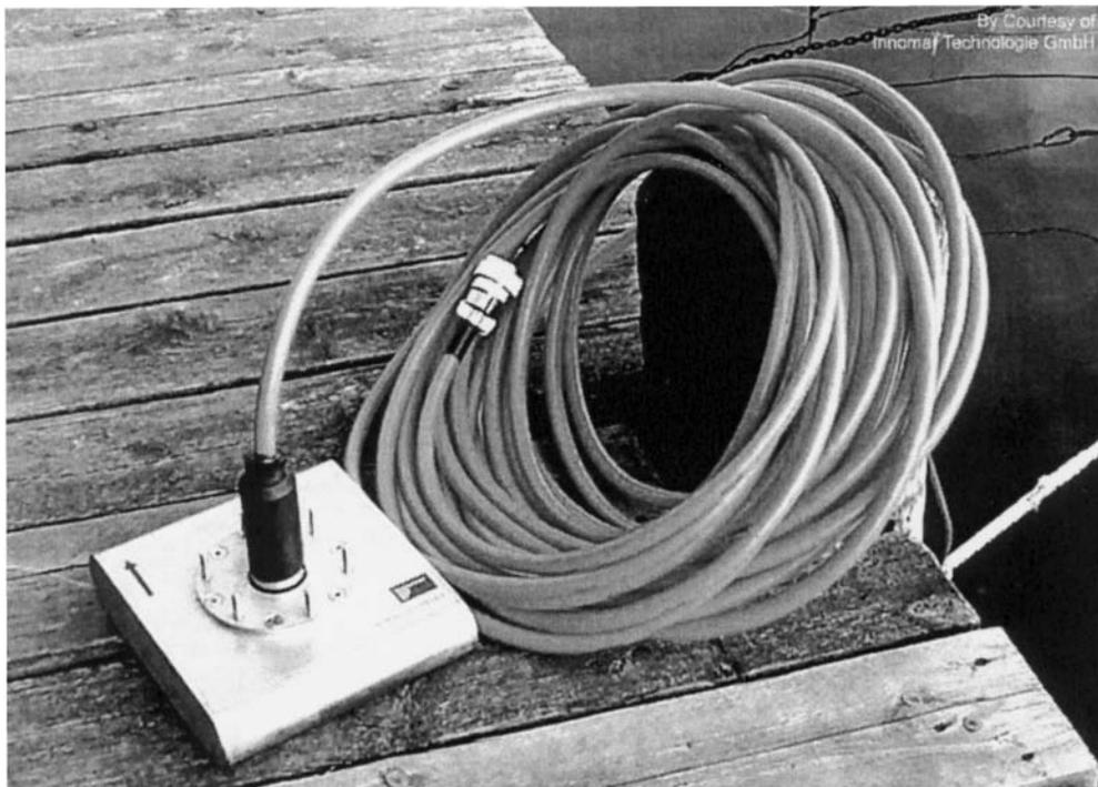
Figure 134: Innomar SES 2000 Compact - parametric transducer with cable
