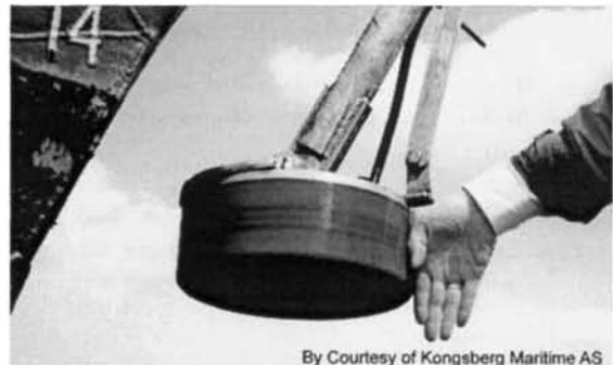
Figure 126: Single beam ceramic transducer
