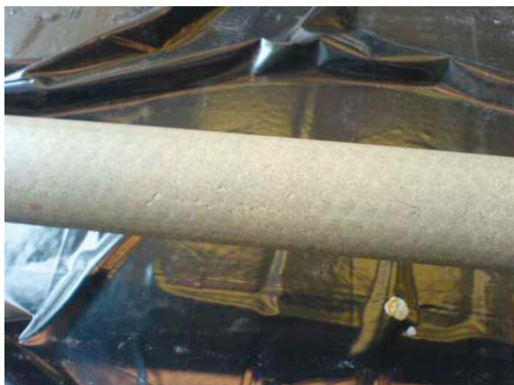
Fig. 4.68 Appearance of “Basic” plug extruded after 3 weeks of maturation. The perforation can be seen through the thin “skin”, which would have become denser and less transparent had the plug have access to water not only at the ends but also over the periphery [12]
