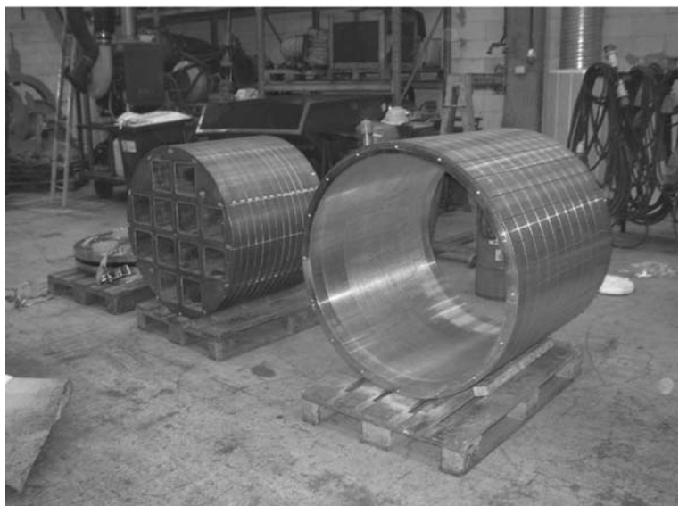
Fig. 3.3 Presently proposed SKB canisters. Upper: Schematic picture of the design. Lower: Iron columns with channels for 12 bunches of spent fuel to the left, and copper liner to the right [1,2]
