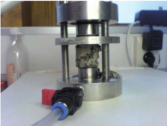
Fig. 2.11 Typical failure with oblique shear planes formed at uniaxial compression of dense clastic clay with a high content of clay particles <2\mu\text{m}
