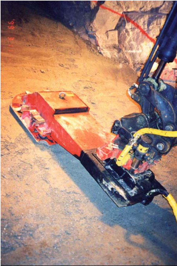
Fig. 4.32 Vibratory plate held and manouvered by a tractor in SKB's slope compaction tests [13]
