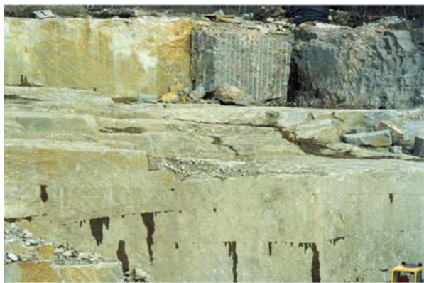
Fig. 2.8 Quarry in granite showing the typical orthogonal pattern of high-order discontinuities of granite: two sets of steep ones and one subhorizontal with water flowing in channels. The platform resulted from a subhorizontal thin 3rd order discontinuity
