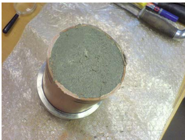
Fig. 4.30 Tube with MX-80 pellets embedded in mud of 50/50 MX-80 and silica flour sectioned after 40 days of exposure to tap water flowing around the tube surface at a rate of 50 mm/s. The plug appears to be very homogeneous and the pellets can hardly be discerned
