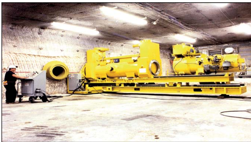
Fig. 4.39 Simulated disposal of RH-TRUW canisters in WIPP [22] (By Courtesy of US EPA)
