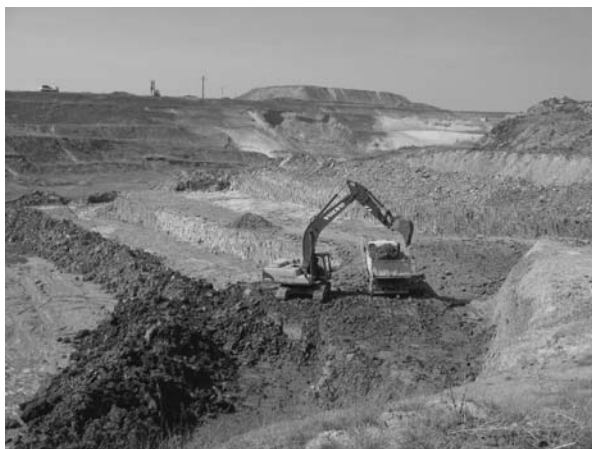
Fig. 1.7 Mining of Tertiary clay (Friedland Ton) in Germany (Photo: Frieton AG)
