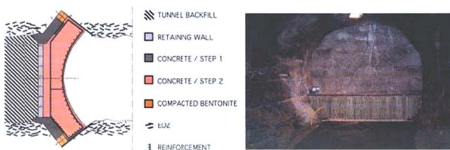
Fig. 4.5 Permanent plug (“Permplug” in Fig. 4.2) of concrete cast on site in two steps for minimizing thermally induced strain. The plug shown was constructed at about 400 m depth in crystalline rock and leaked despite the careful construction work [3]
