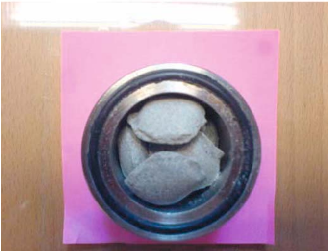
Fig. 4.71 Pellet fill. Upper : Schematic picture of the microstructural constitution; the grains take up water from the boundaries by which they expand and give off clay particles that form gels in the voids between the expanded grains. Lower : Pellets with 10% water content in 30 mm cell
