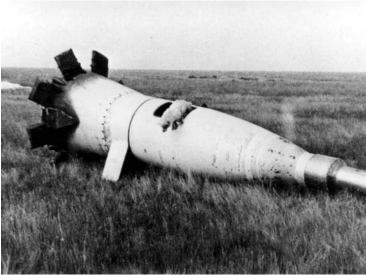
A dog exits her capsule in the nose section of an R-2A rocket. Note the scorch marks on the air brakes, which were used to slow the capsule before deployment of the parachute. (Photo: authors' collection)
