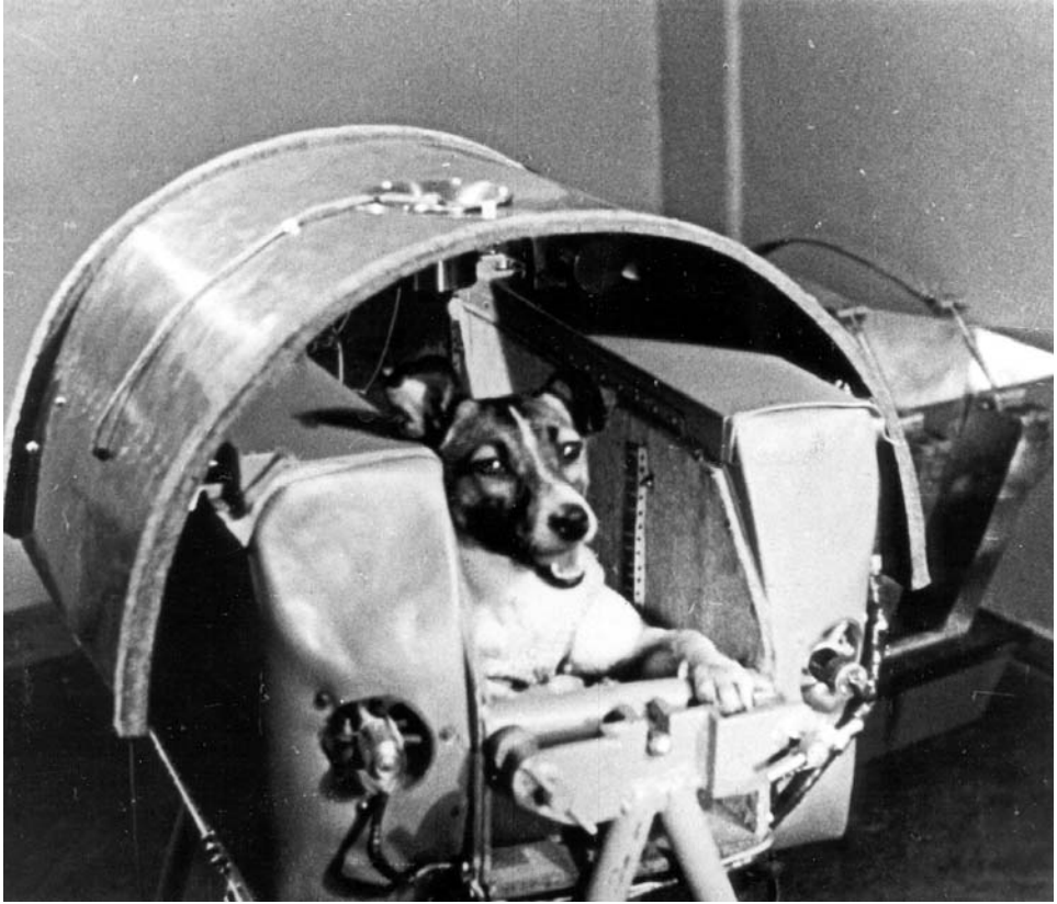
Tucked into place between her cushions and beneath the insulated heat shield, Laika was ready to be loaded into her capsule. (Photo: authors' collections)
