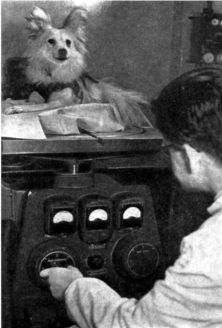
To familiarise them with the vibration they would experience during a rocket launch, dogs were trained on a vibration table such as this one. (Photo: authors' collections)
