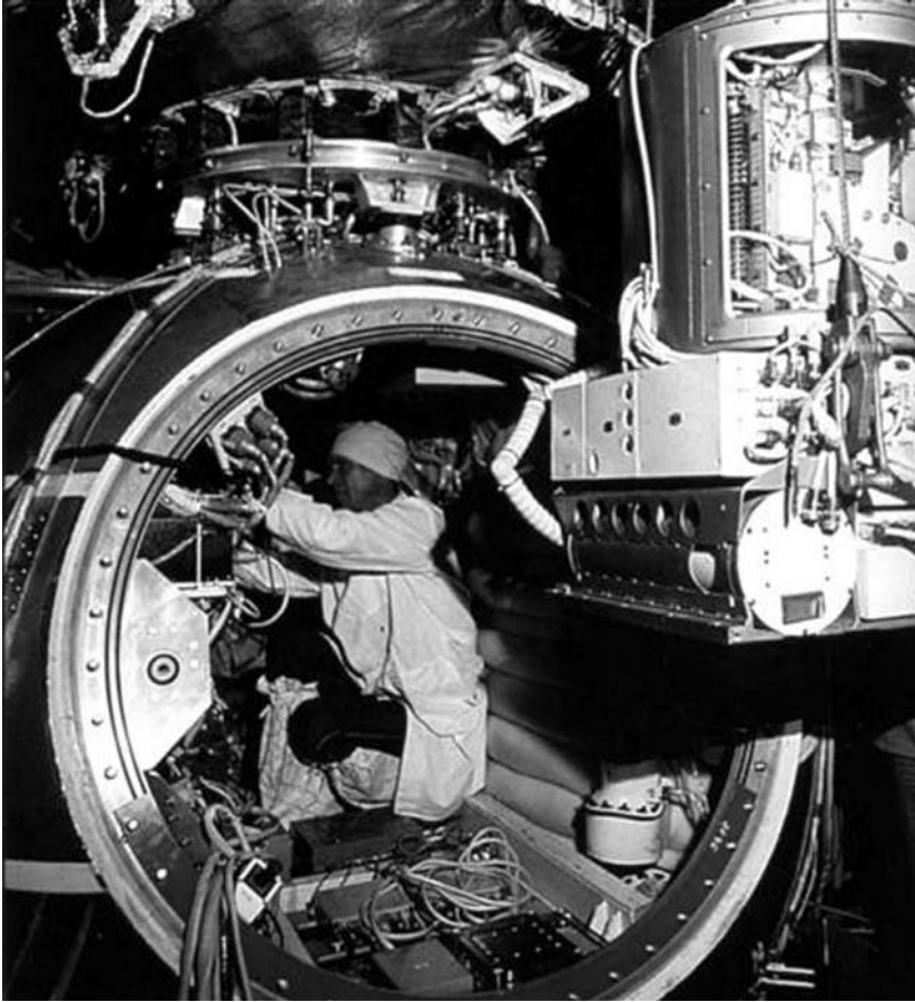
A Russian technician works inside the payload section of the Cosmos/Bion spacecraft. (Photo: authors' collections)
