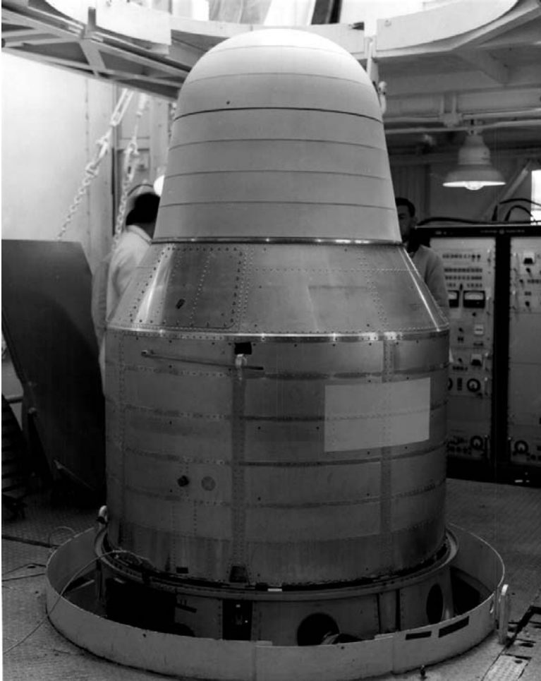
Biosatellite 1 spacecraft mated to a Delta booster with cover off. (Photo: NASA-KSC)
