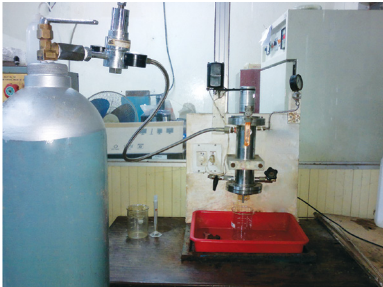
Plate 7.1 Stirred batch cell set-up.
