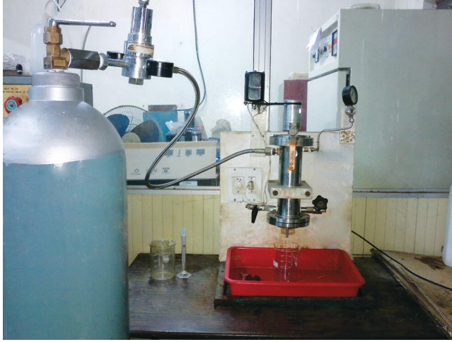
Figure 7.12 Stirred batch cell set-up. For a colour version of this figure, see Plate 7.1.
