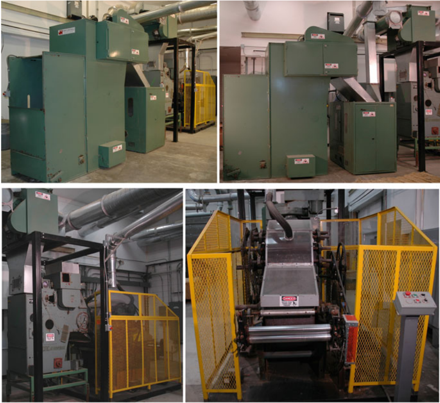
Fig. 3.2 Flax Cottonizing Line fiber blender and opener that takes fiber tufts and continually opens them into smaller and lighter tufts for the pin beater ( top left ). Flax Cottonizing Line pin beater for fine flax fiber separation and cottonizing ( top right ). Flax Cottonizing Line card-evenfeeder forms a consistent mat of fibers that when delivered to the card has an even mass in longitudinal and lateral directions, well opened, and delivered in a consistent manner ( bottom left ). Flax Cottonizing Line rollertop card contains card cylinder along with “workers” and “strippers” to help open tufts, orient fibers, and remove short fibers, neps, dust, and trash ( bottom right )
