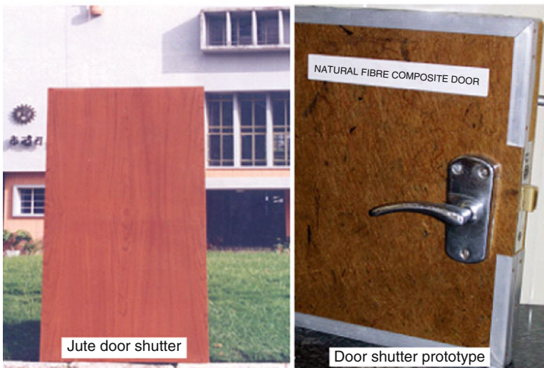
Fig. 24.5 Jute sandwich panels and door shutter
