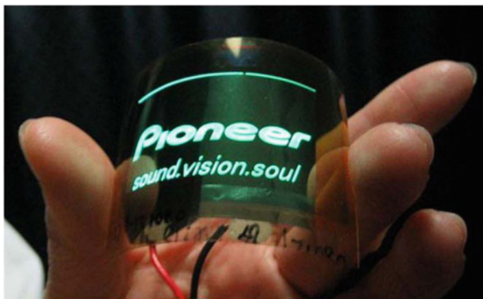
Fig. 21.6 Luminescence of an organic light-emitting diode deposited onto a flexible, low CTE and optically transparent wood–cellulose nanocomposite. Reproduced with permission from Okahisa et al. (2009). Copyright © 2009, Elsevier Ltd
