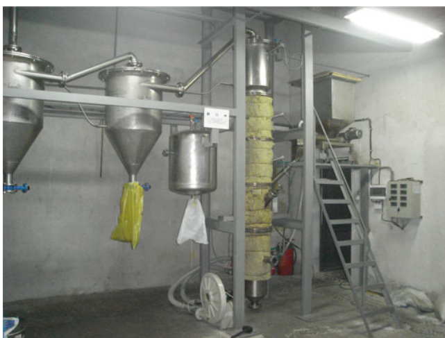
Fig. 13.6 A photograph of the pilot plant for rice husks pyrolysis
