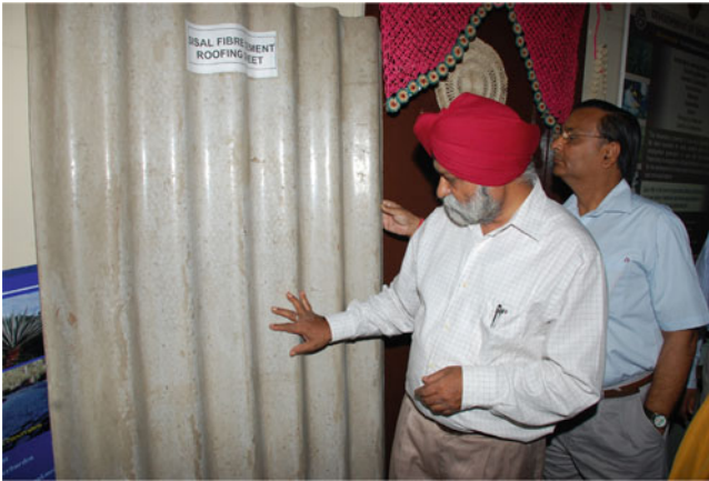
Fig. 22.8 Sisal fiber cement roofing sheet
