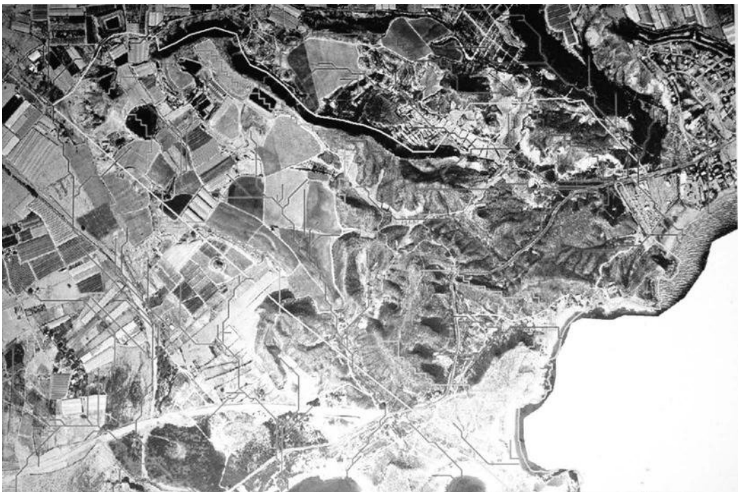
FIGURE 22.7 Identification of the drainage network.
