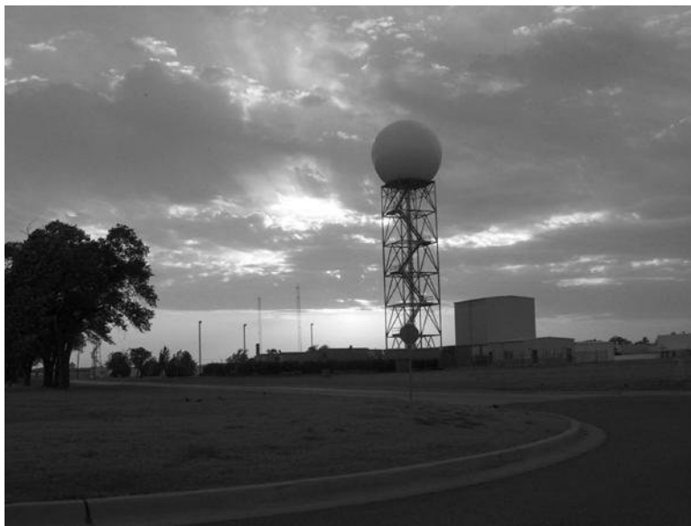
FIGURE 21.3 A WSR-88D radar dome at the NWS Radar Operations Center in Norman, Oklahoma.
