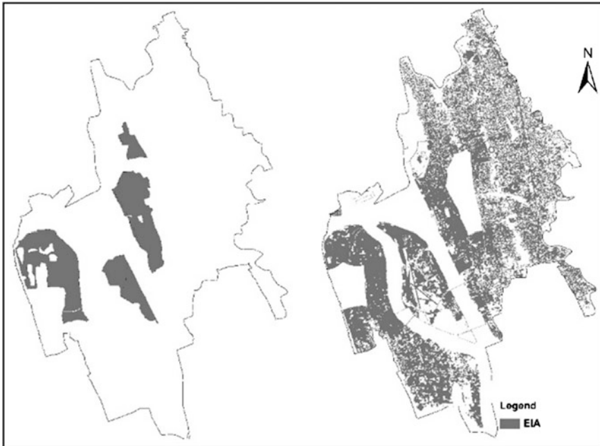
Fig. 5 Land use changes in the study area for last 42 (1968–2010) years in terms of effective impervious area (EIA)
