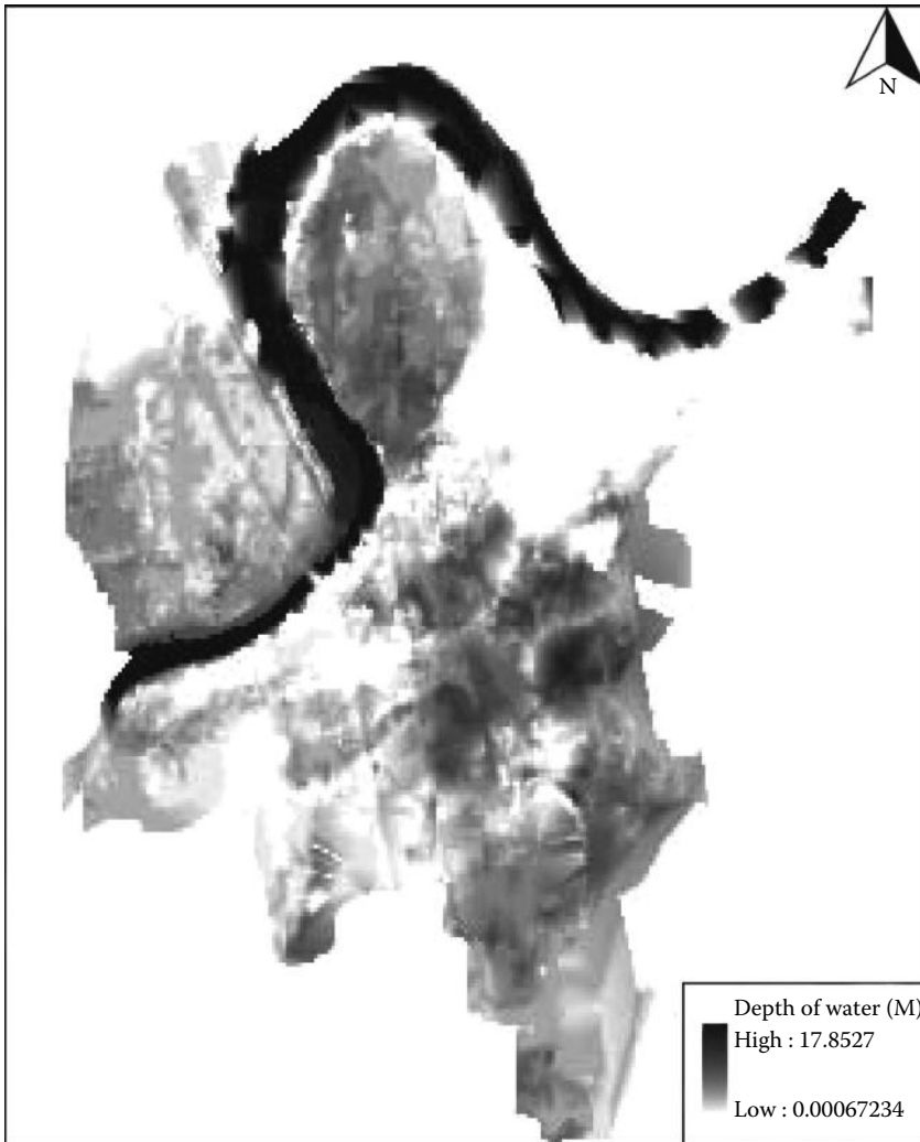
FIGURE 12.4 Flood depth map of study area after diversion of 2,832 m 3 /s of floodwater.
